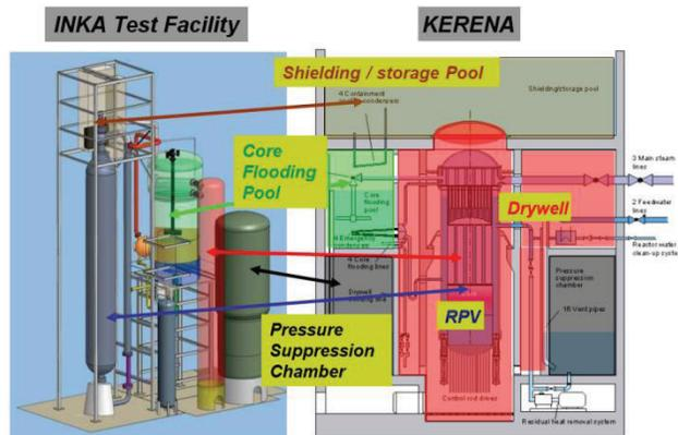
**Figure 2: Comparison between the KERENA Containment and the INKA test facility.**
