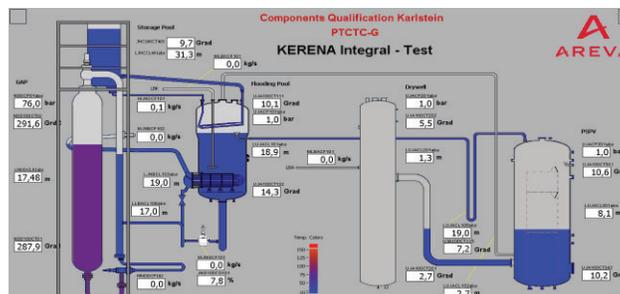
**Figure 5: Online P&ID, showing real-time test data (INKA control room view).**
