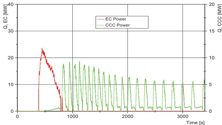
**Figure 7: EC and CCC heat transfer capacity as function of time.**
