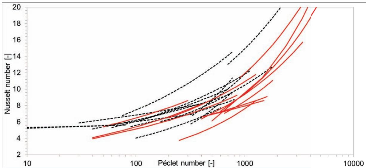
Figure 4 Comparison between alkali metals (broken black curves) and heavy liquid metals (solid red curves)
