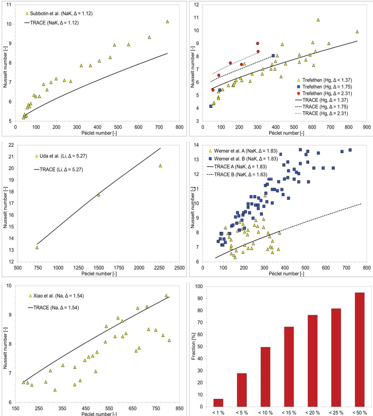
Figure 7 Experimental and predicted Nusselt number as a function of the Péclet number for various experiments (cont.) and fraction of the data points within a certain range (bottom right)
