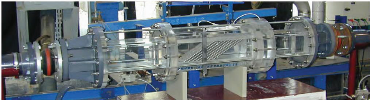
Figure 1. EOLE test section with a tube bundle inclined at 30^\circ .
