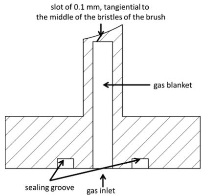
**Figure 5. Section Through the Gas Inlet Nozzle.**
