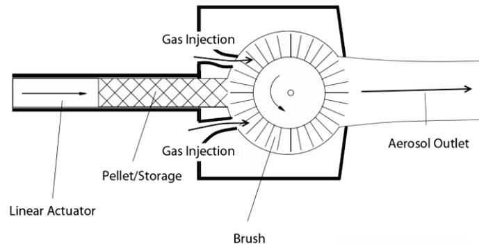
**Figure 4. Functional Principle of the PDB.**
