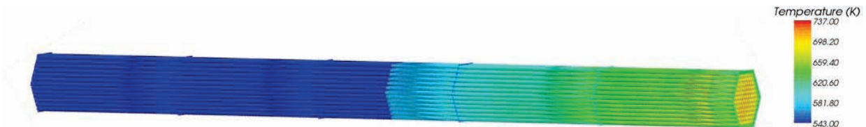
Figure 13. Temperature distribution in the MYRRHA fuel assembly under nominal conditions.
