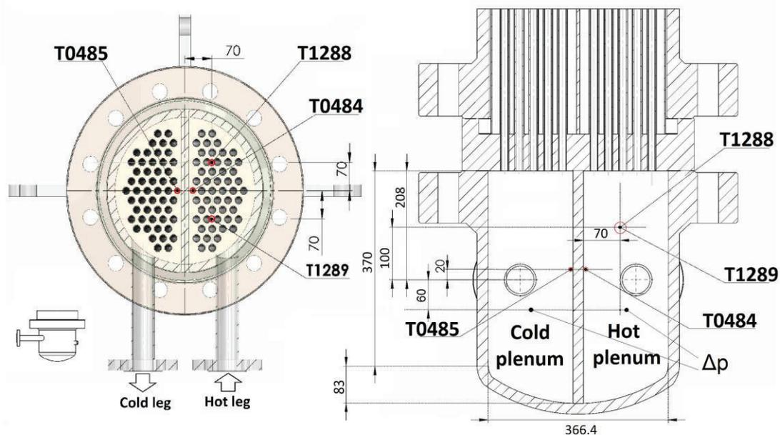
Figure 2. The temperature and pressure measurements in the hot and cold plenum in the PWR PACTEL steam generator 2.
