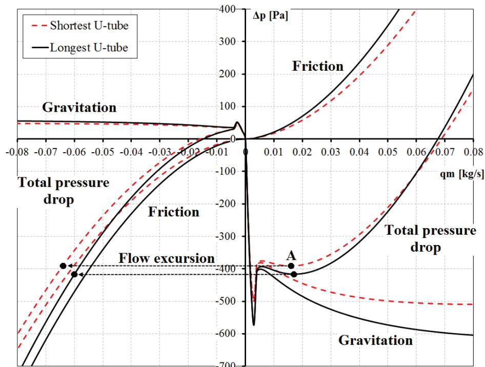
Figure 4. The total pressure drop and the friction and gravitation pressure drops as a function of mass flow in the shortest and the longest U-tube of the PWR PACTEL steam generator in the conditions of RF-02 experiment and at the uniform inlet temperature of 245 °C (average temperature of hot plenum).
