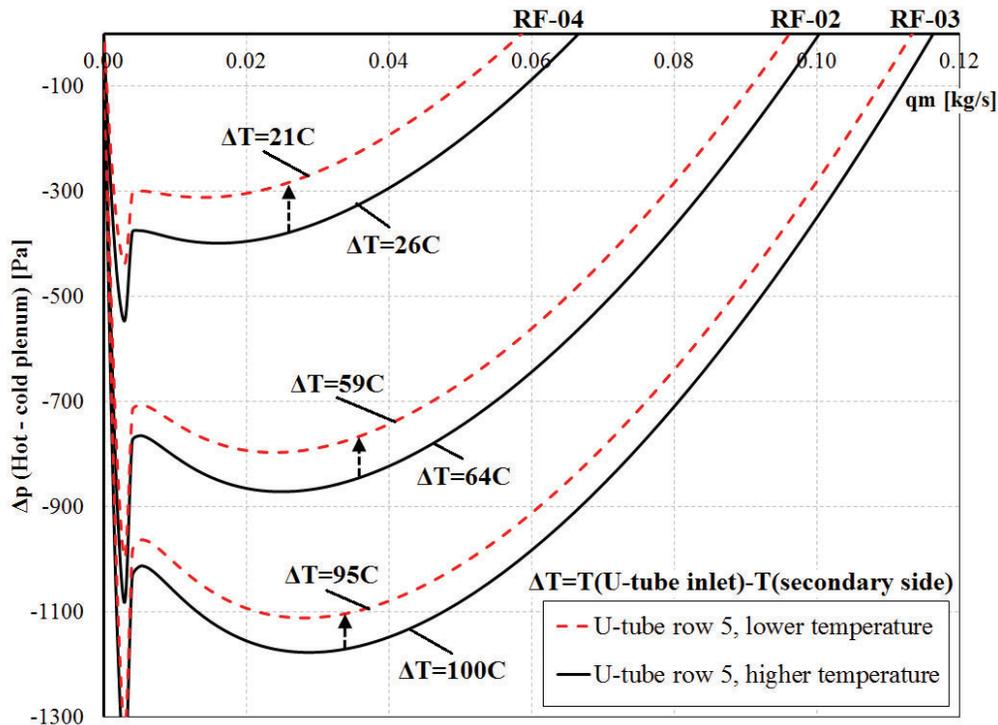
**Figure 6. The characteristic curves for the medium length U-tube with different inlet temperatures in the conditions of the experiments RF-02, RF-03, and RF-04. Notice that with lower inlet temperature, the flow in the U-tube is less stable enabling the flow reversal in it more easily.**
