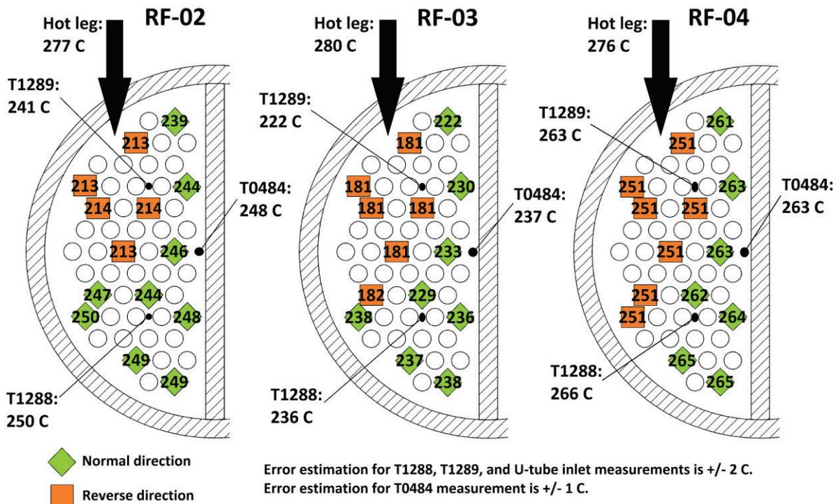
Figure 3. Flow direction and measured temperatures inside the instrumented U-tubes and the hot plenum of steam generator 2 in the experiments RF-02, RF-03, and RF-04. The black arrow indicates the flow direction from the hot leg. The U-tube temperatures are measured at the level of 0.3 m with the exception of the U-tubes 22 and 43 in which they are extrapolated from the level of 0.7 m.
