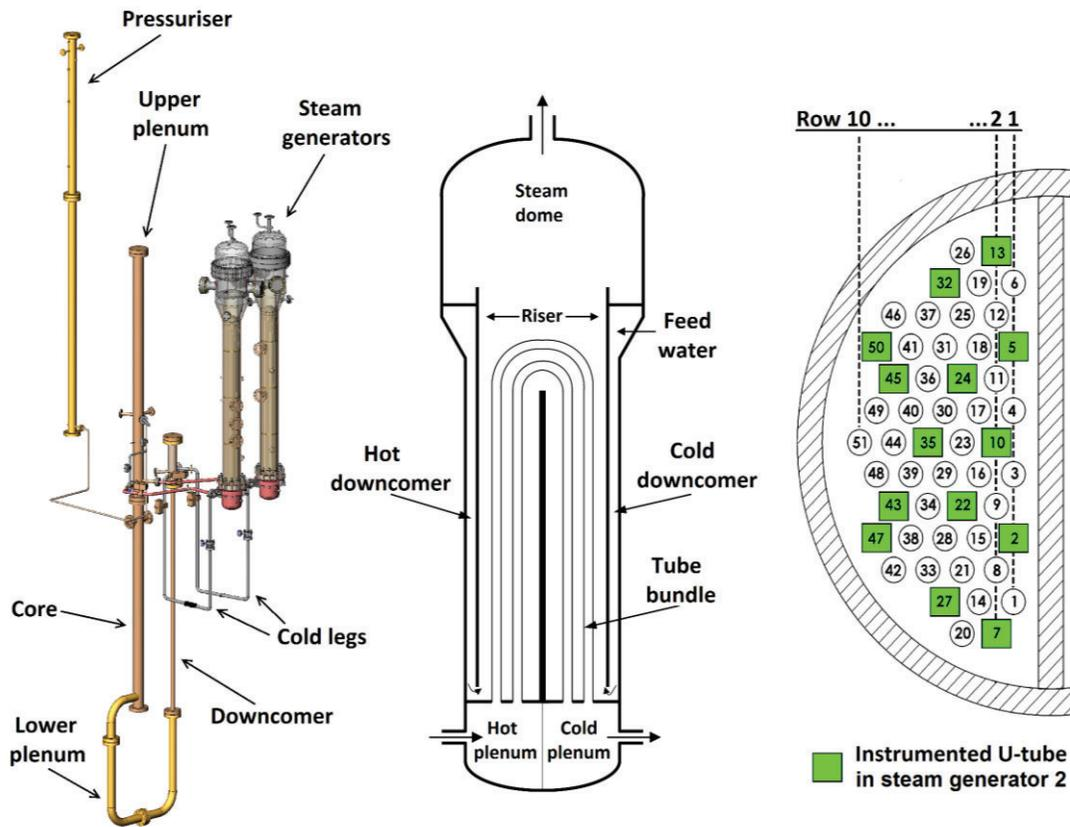
Figure 1. The general view of the PWR PACTEL facility, the schematic view of the PWR PACTEL steam generator, and the arrangement of the U-tube bundle.
