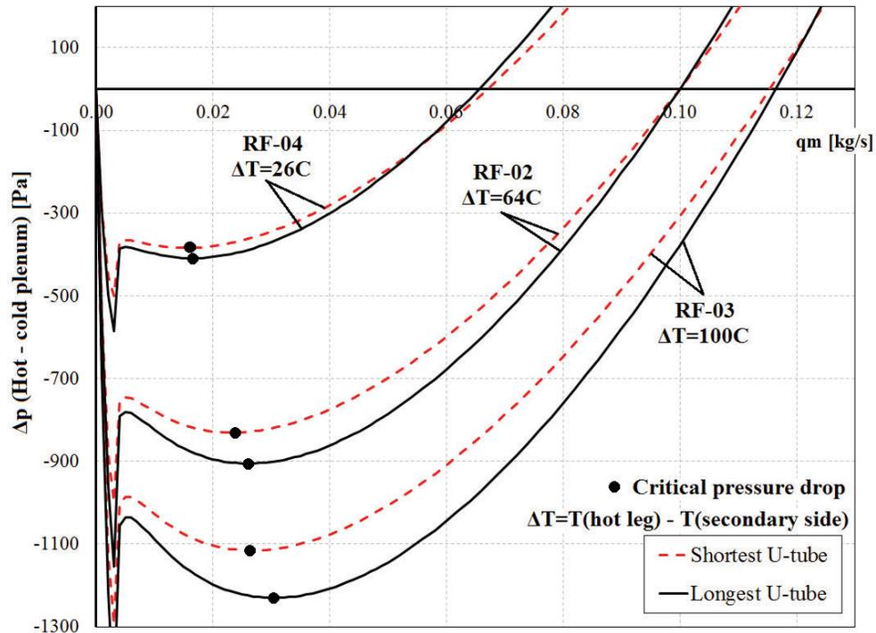
Figure 5. The characteristic curves for the shortest and the longest U-tube in the conditions of the experiments RF-02, RF-03, and RF-04 and at the uniform inlet temperature (hot leg temperature) of 277 °C, 280 °C, and 276 °C, respectively. According to these characteristic curves, the short U-tubes should have been reversed, whereas in the experiment reversed flow was observed in the long U-tubes.
