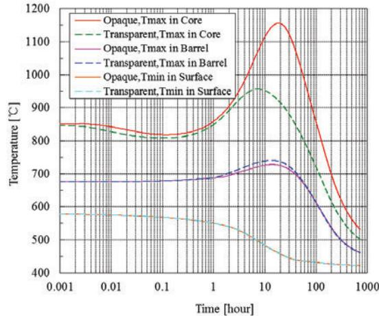
**Figure 2 The top temperatures in the core, the barrel and the surface of the reactor body vary with time, with regarding the influence of the molten salt radiation performance on the temperature.**
