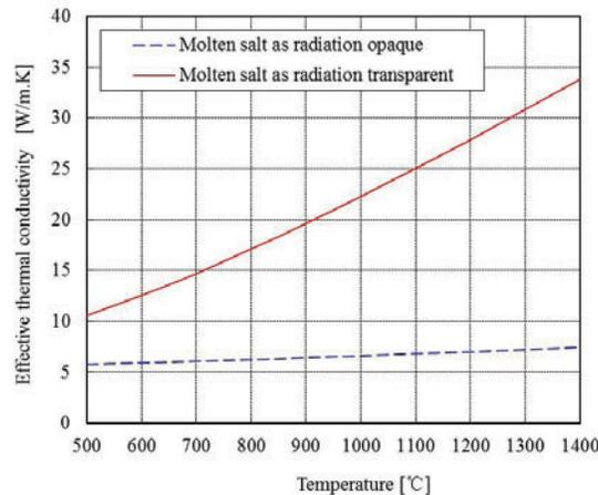
Figure 1 Effective thermal conductivity vary with temperature
