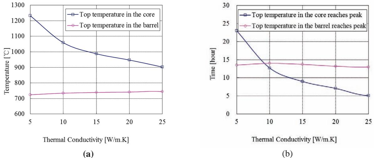
**Figure 3 The peak temperature in the core and the barrel and their corresponding time after reactor shutdown vary with the effective thermal conductivity**
