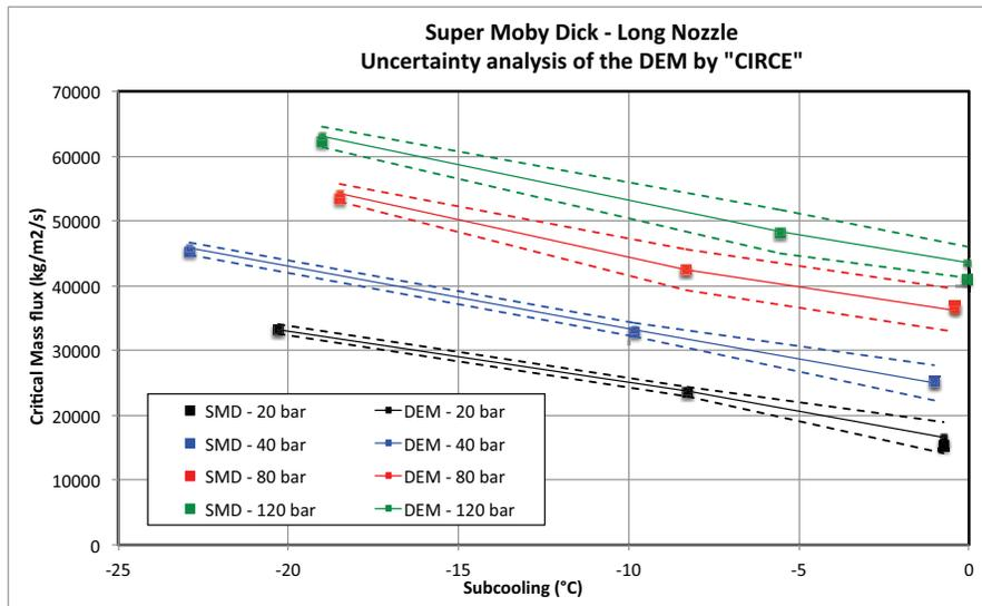
Fig. 5: Uncertainty evaluation of the DEM model on the Super-Mobydick long nozzle
