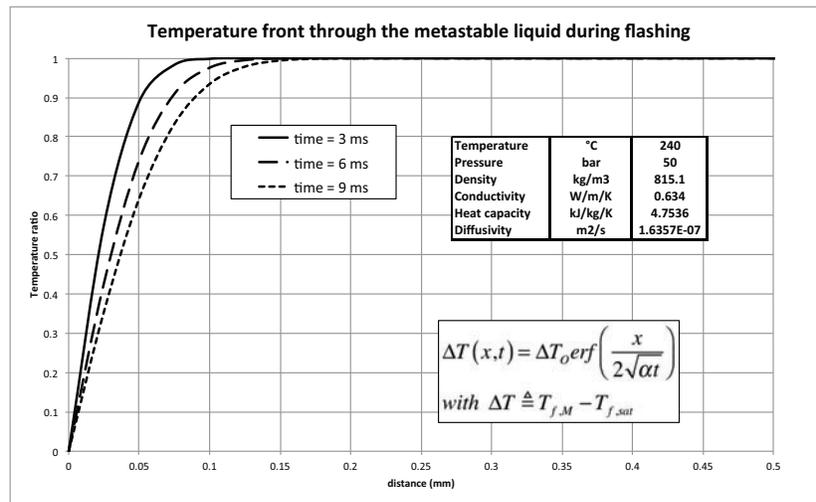
Fig. 2 Temperature profiles in the metastable liquid
