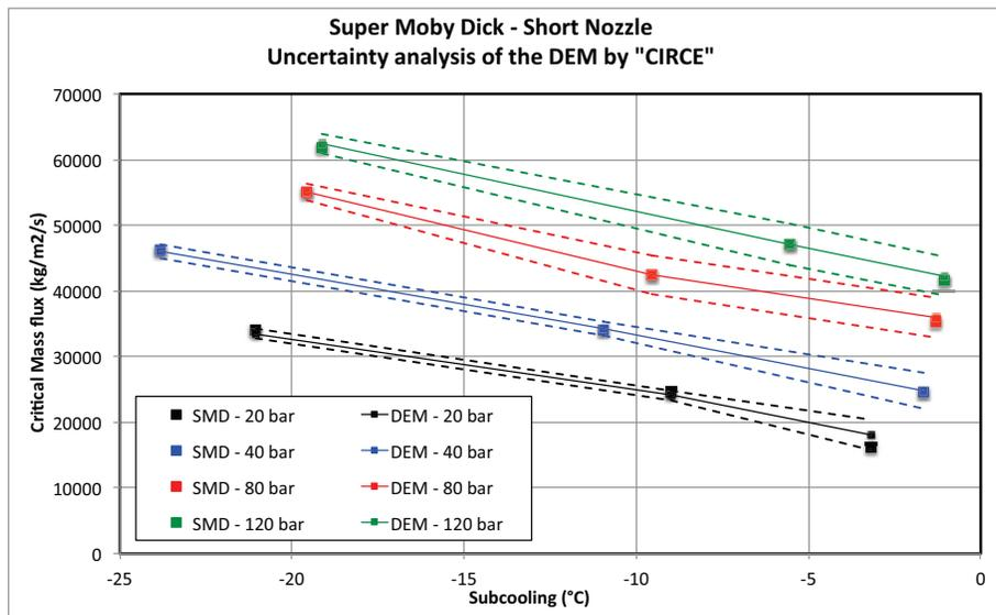
Fig. 4: Uncertainty evaluation of the DEM model on the Super-Mobydick short nozzle
