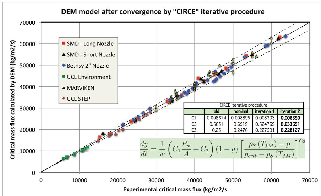
Fig 3. Comparison between experimental critical mass flux and DEM calculation - Dashed lines +/- 5%
