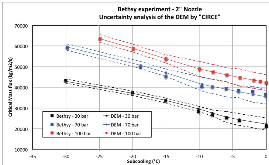
Fig. 6: Uncertainty evaluation of the DEM model on the Bethsy 2" nozzle
