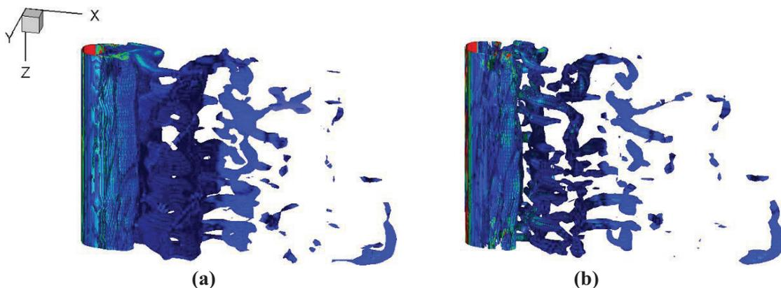
Figure 4. Contours of instantaneous vortex structure for  $\alpha = 0^\circ$ ,  $A=9$  and  $T^*=450$ : (a)  $|\omega| > 50 \text{ s}^{-1}$ ; (b)  $Q = 1000 \text{ s}^{-2}$ .
