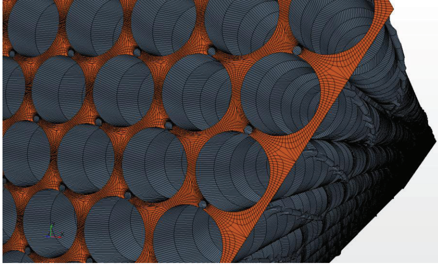
Fig. 8 SFR fuel S/As – 3D CFD meshing of the computational domain
