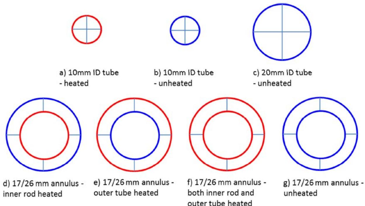
Figure 1. Cross-sectional Schematic of Risø Test Tubes and Annulus
