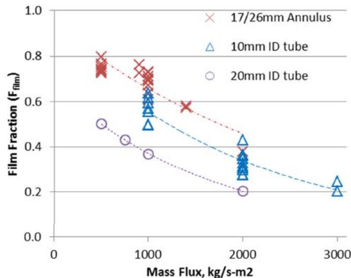
**Figure 3. Measured Film Fraction with Mass Flux**
