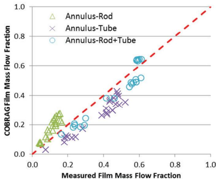
**Figure 5. COBRAG Predicted Film Mass Flow Fraction for Heated Annular Test Section**
