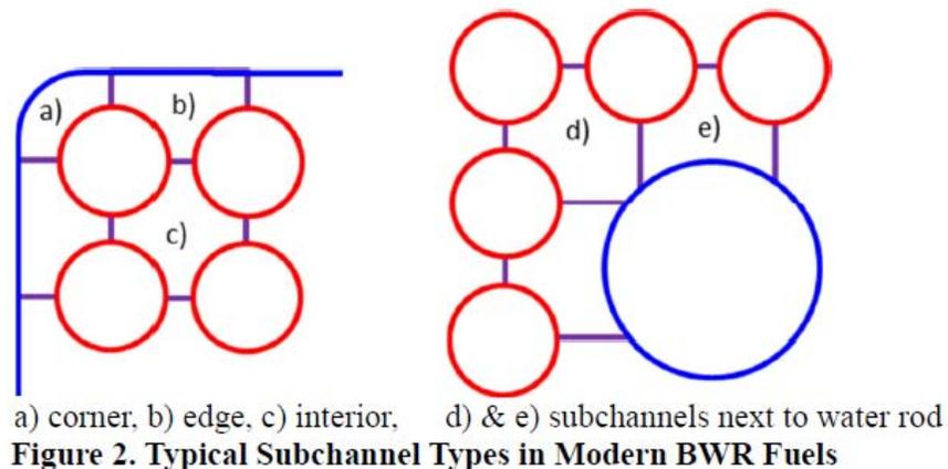
a) corner, b) edge, c) interior, d) & e) subchannels next to water rod
