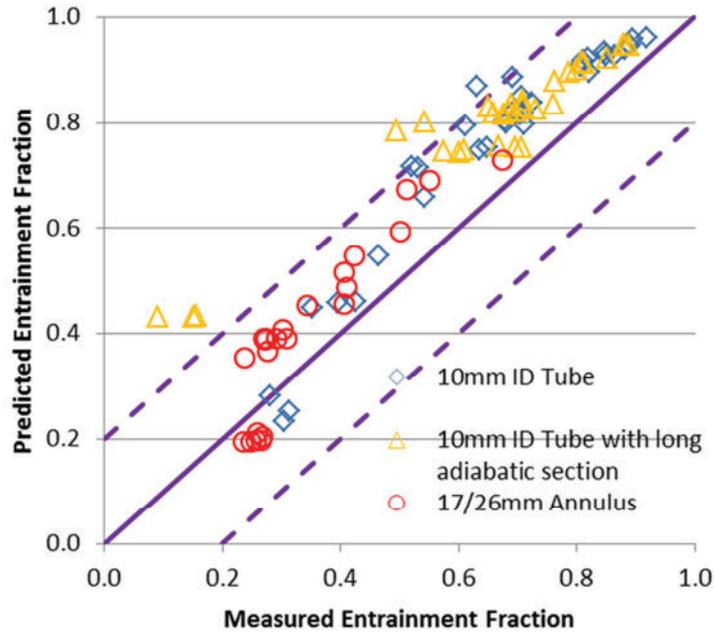
Figure 7. COBRAG Predicted Entrainment Fraction for Heated Annulus/Tube Data
