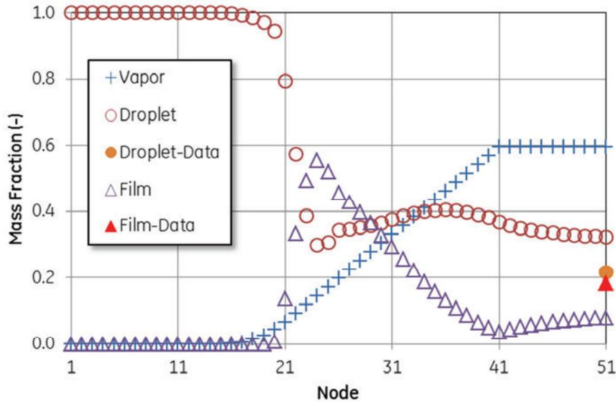
Figure 9. COBRAG Prediction for 10mm Tube data 363
