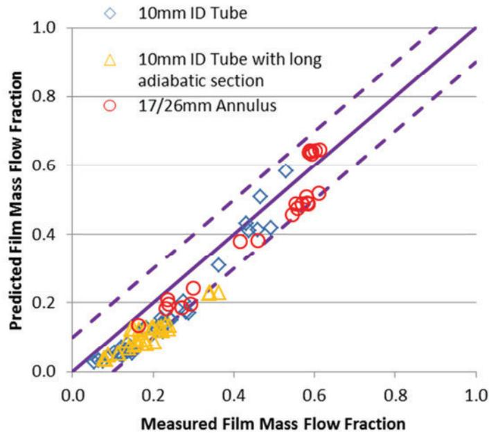
Figure 6. COBRAG Predicted Film Mass Flow Fraction for Heated Annulus/Tube Data
