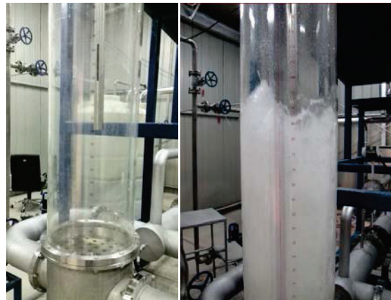
Figure 4. Air Inlet Distributor and Test Section
