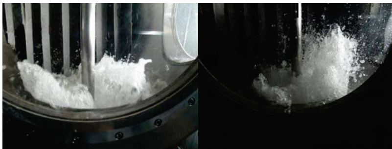
Figure 1. Transition to Pseudo Jet/Fountain Flow at High Gas Flux Conditions
