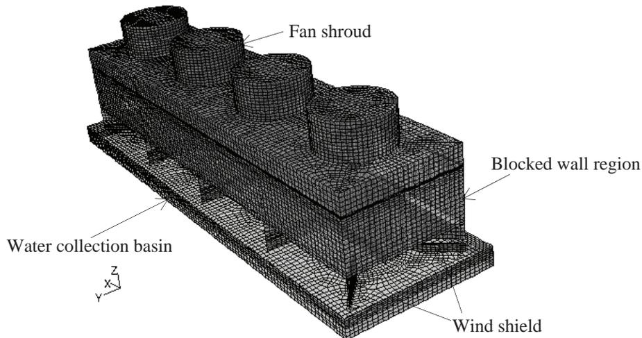
**Figure 2. Computational meshes for the three-dimensional domains representing H-area countercurrent flow MDCT ( $2.5 \times 10^6$  meshes)**
