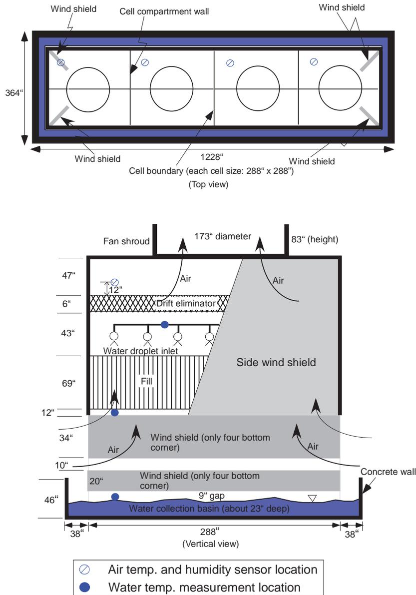
**Figure 1. Top-down view and cross-section view of the compartment cell instrumented for the performance measurement for H-area cooling tower (1" = 0.0254 m).**
