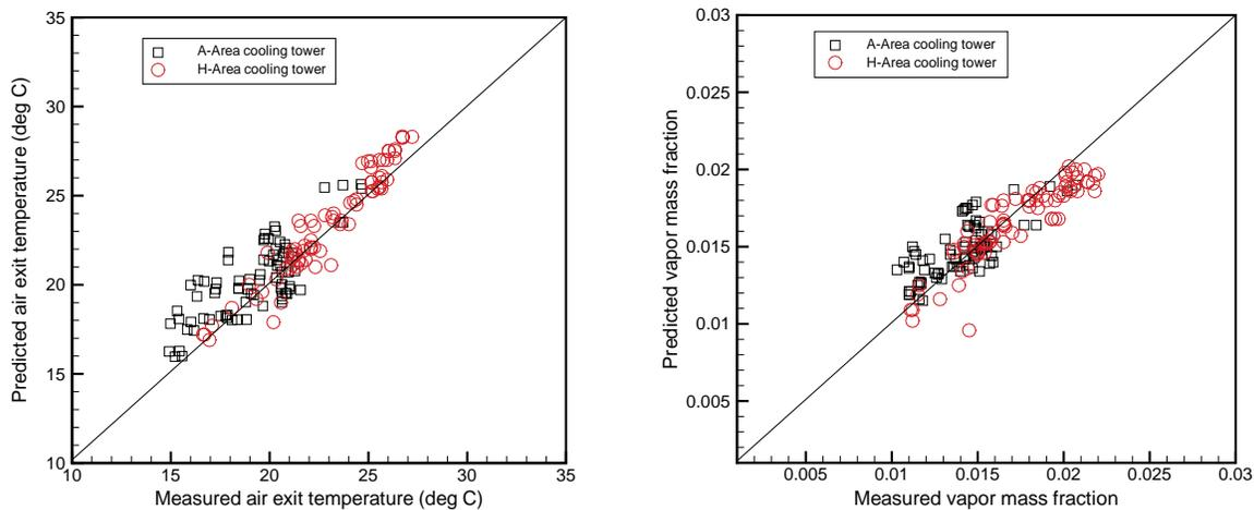
**Figure 3. Comparison of the modeling predictions with the measured air exit results for A-Area (cross-flow) and H-Area (countercurrent flow) cooling towers**
