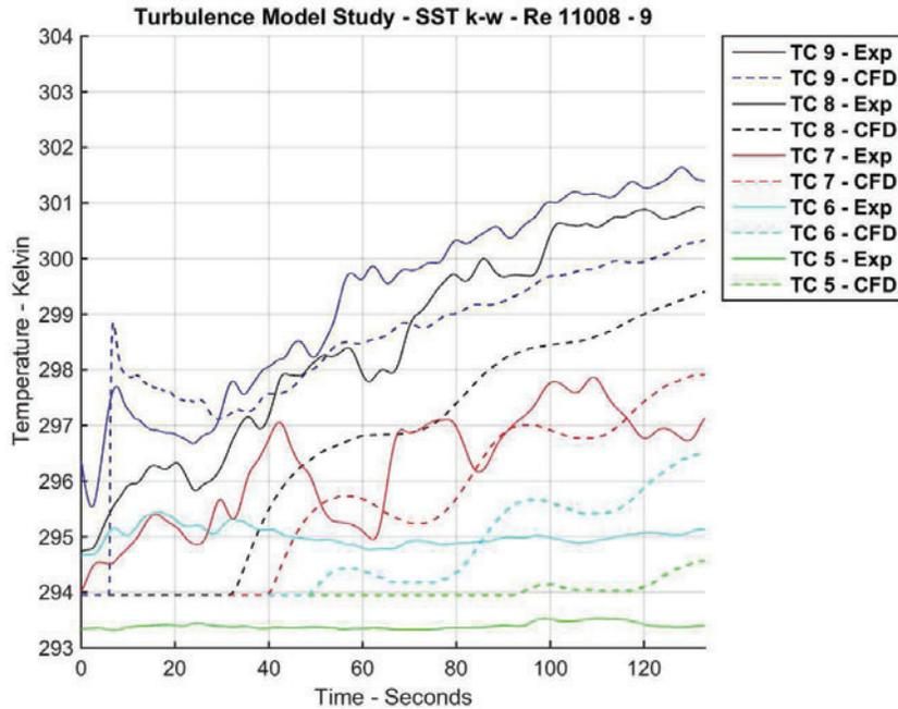
**Figure 7. Comparison of Experimental and Simulation Temperature Traces - SST.**
