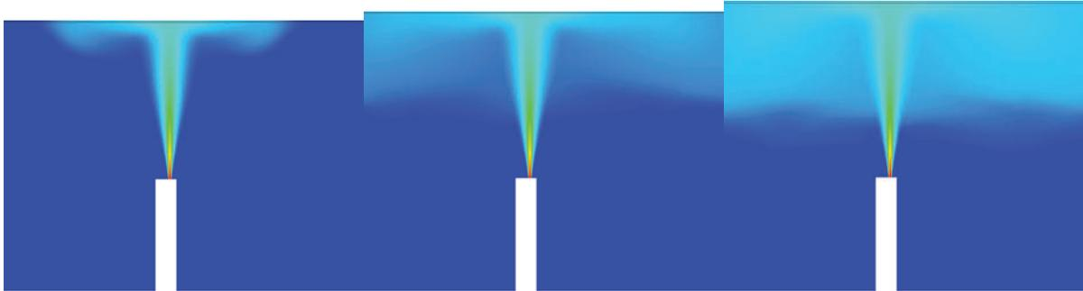
Figure 11. Evolution of Temperature Field for the Standard Low-Reynolds  $\kappa$ - $\epsilon$  Simulation at 8, 65 and 130 Seconds
