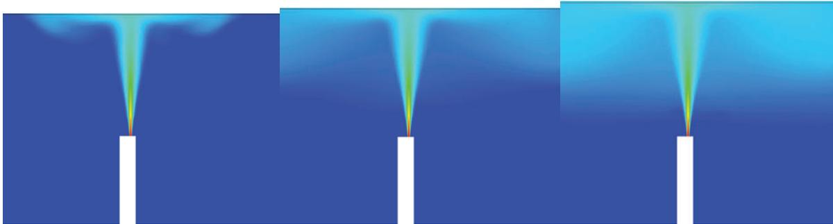
Figure 13. Evolution of Temperature Field for the Shear Stress Transport  $\kappa$ - $\omega$  Simulation at 8, 65 and 130 Seconds
