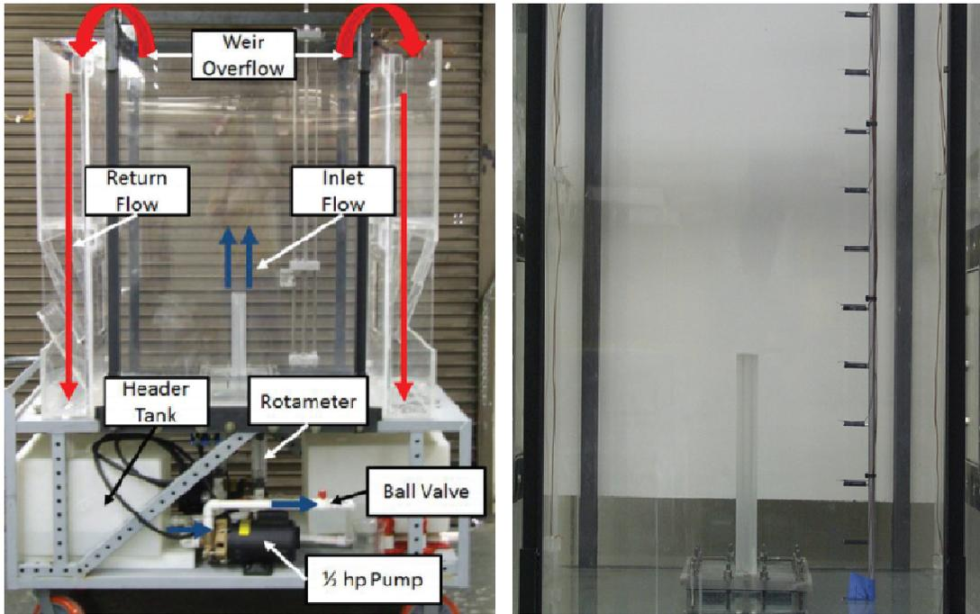
**Figure 1. Twin Jet Water Facility and Measurement Instrumentation for Thermal Stratification Studies**
