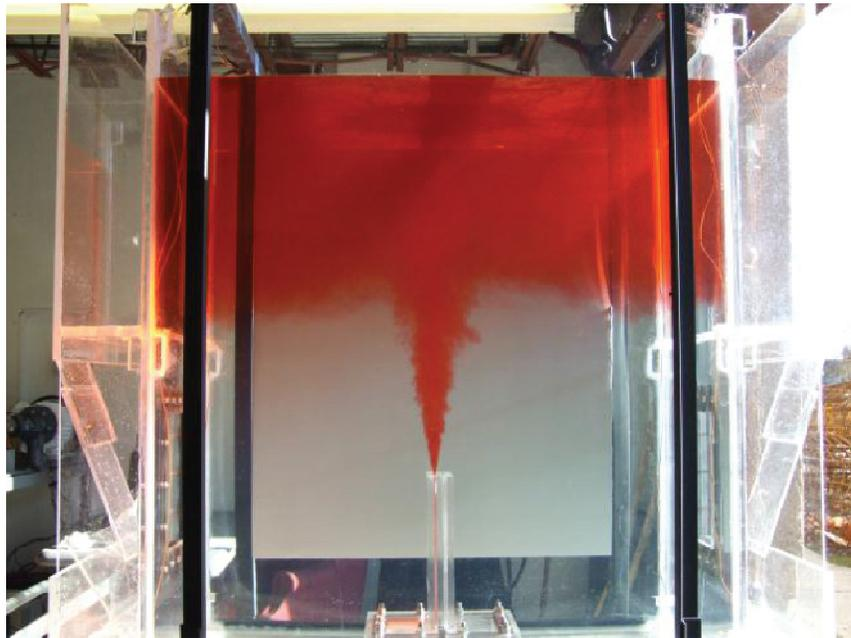
**Figure 2. Initial Trial showing Thermal Stratification within the TJWF**
