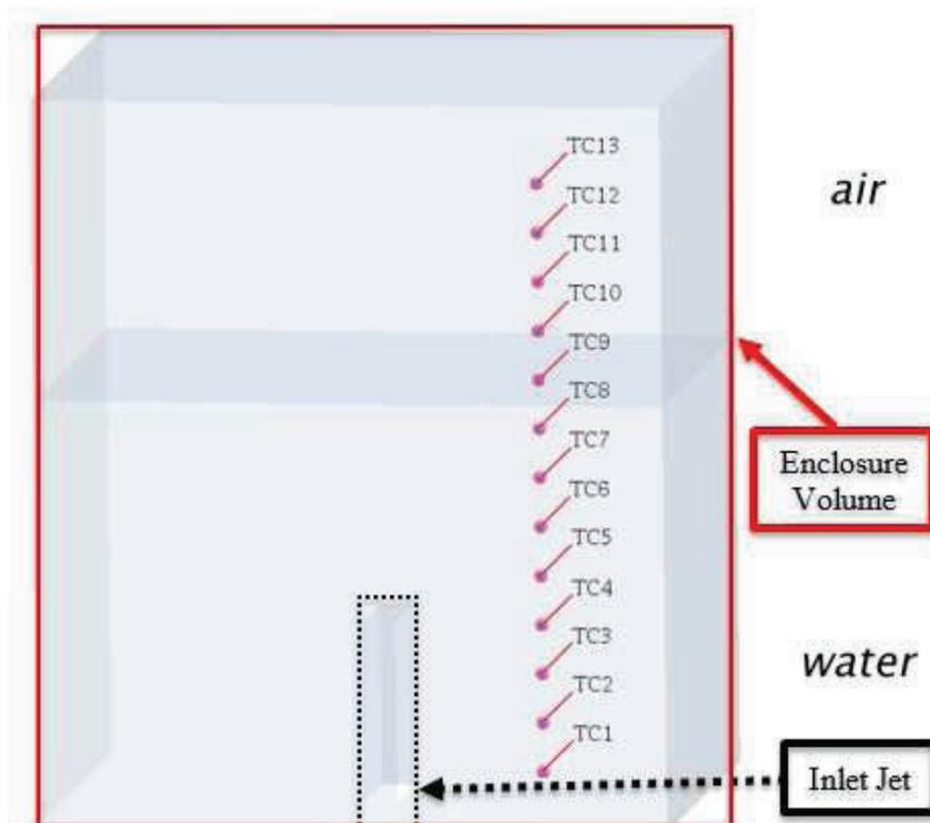
**Figure 3. Division of the TJWF Computational Domain and Temperature Probe Locations**
