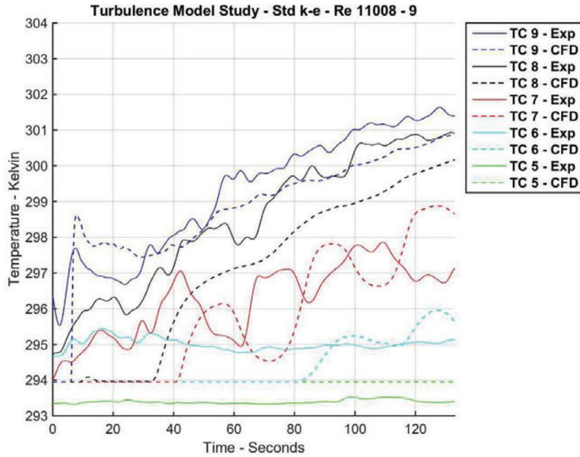
Figure 5. Comparison of Experimental and Simulation Temperature Traces Standard Low - Reynolds  $\kappa\text{-}\epsilon$ .
