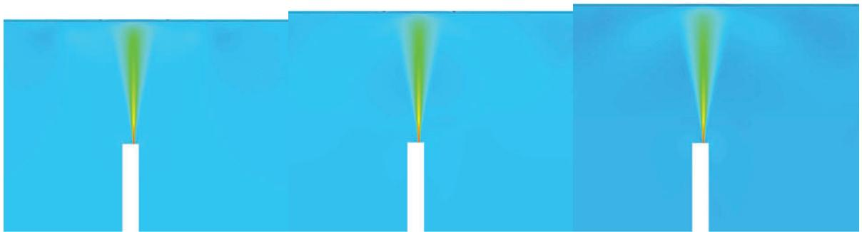
**Figure 10. Evolution of Velocity Field for Shear Stress Transport  $\kappa$ - $\omega$  Simulation at 8, 65 and 130 Seconds**
