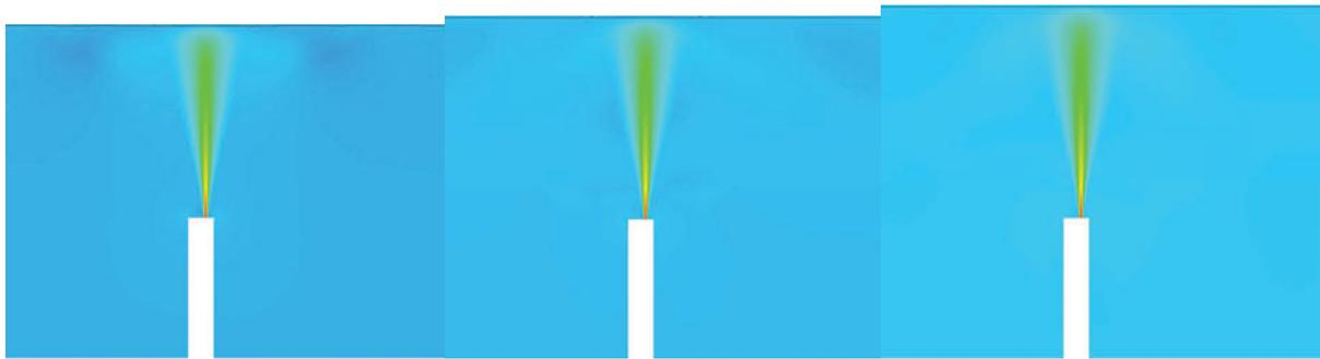
**Figure 8. Evolution of Velocity Field for the Standard Low-Reynolds  $\kappa$ - $\epsilon$  Simulation at 8, 65 and 130 Seconds**
