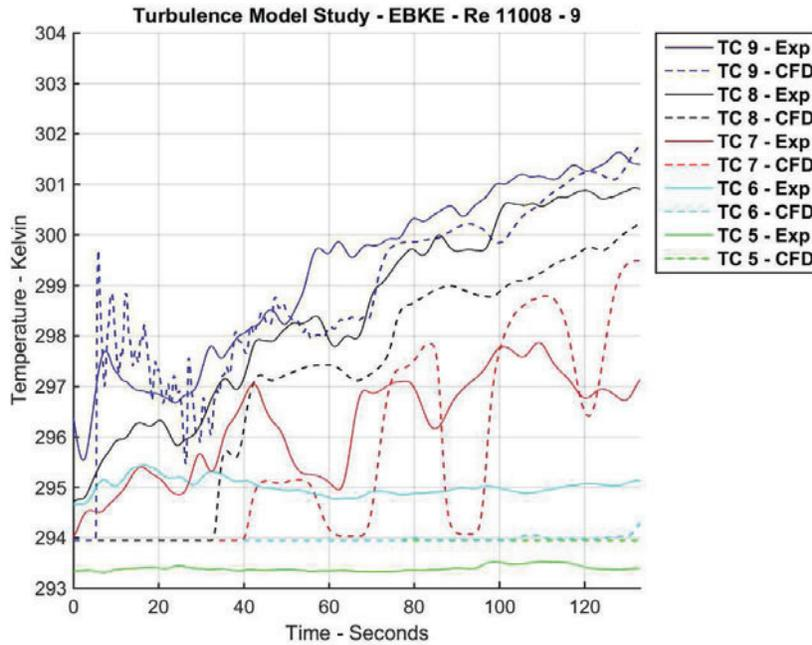
Figure 6. Comparison of Experimental and Simulation Temperature Traces - EBKE.
