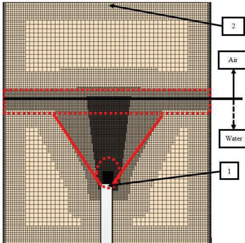
**Figure 4. Mesh and Boundary Conditions for the Enclosure Volume, Jet Outlet – Dotted Oval, Jet Spreading Region – Solid Lines, Water Level Region – Dotted Rectangle**
