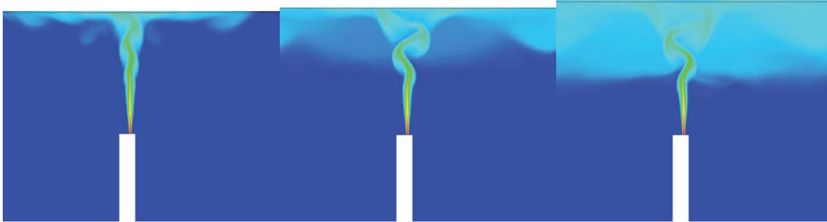
Figure 12. Evolution of Temperature Field for the Elliptic Blending  $\kappa$ - $\epsilon$  Simulation at 8, 65 and 130 Seconds
