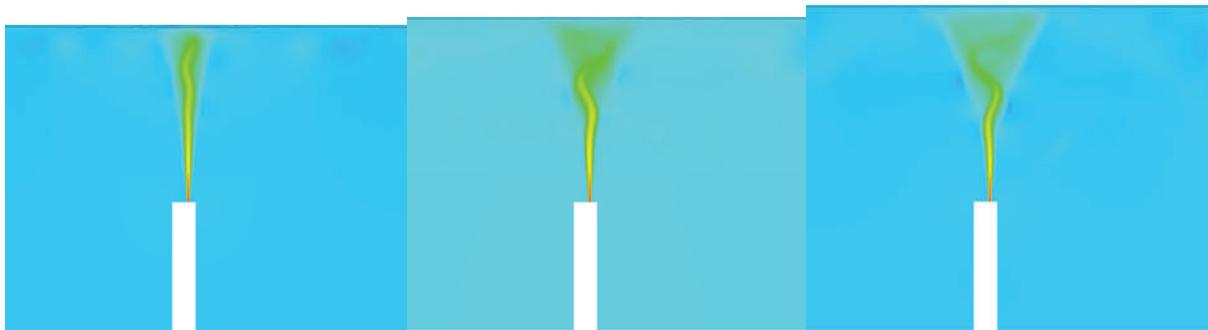
**Figure 9. Evolution of Velocity Field for Elliptic Blending  $\kappa$ - $\epsilon$  Simulation at 8, 65 and 130 Seconds**
