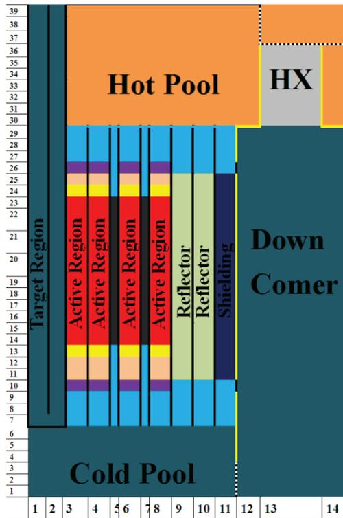
**Fig. 3** Calculation model of the 10 MW<sub>th</sub> ADS
