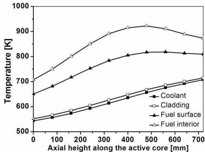
Fig. 5 Axial temperature distributions in the hottest channel of steady state
