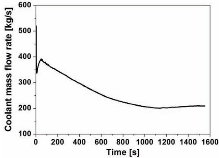
Fig. 8 Coolant mass flow rate in ULOHS
