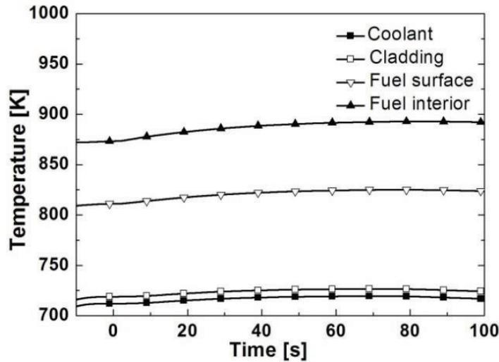
Fig. 13 Temperatures in the hottest channel in UTOP
