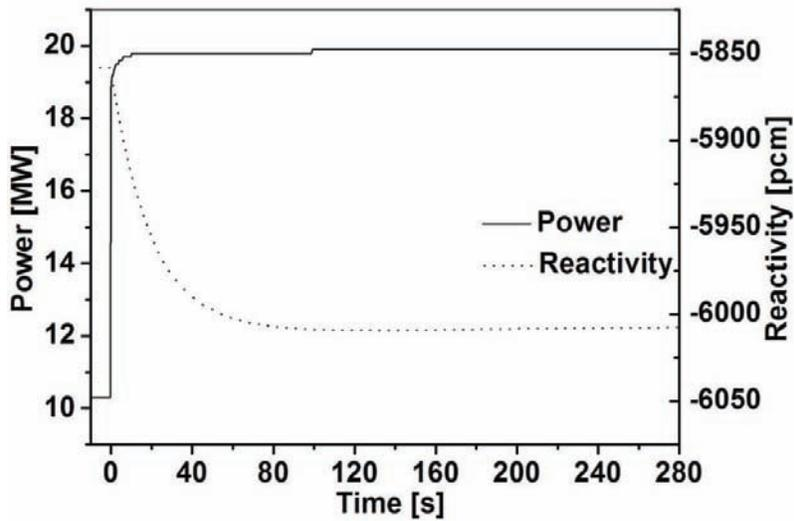
Fig. 9 Core power and reactivity in UBOP
