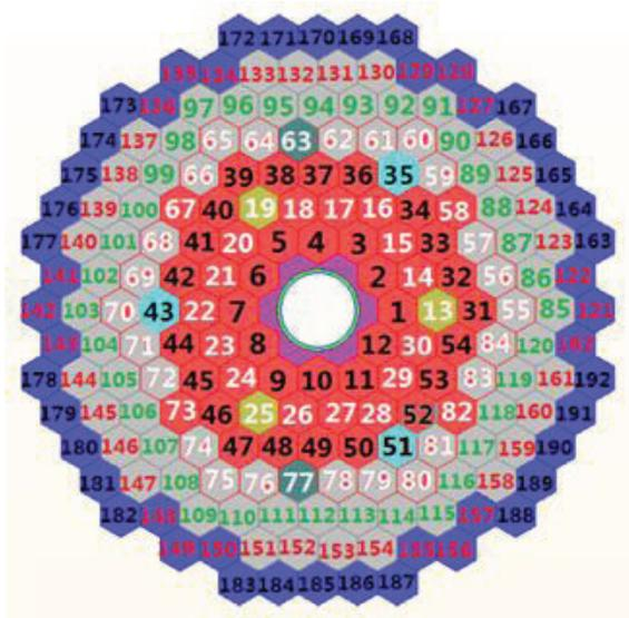
Fig. 2 Core Assembly Distribution of the 10 MW<sub>th</sub> ADS
