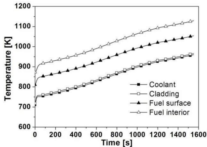
Fig. 7 Temperatures in the hottest channel in ULOHS
