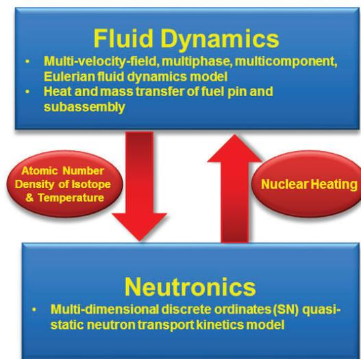
**Fig. 1** The code and function structure of NTC
