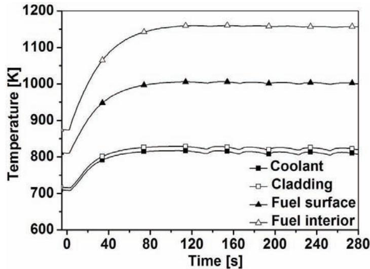
Fig. 10 Temperatures in the hottest channel in UBOP
