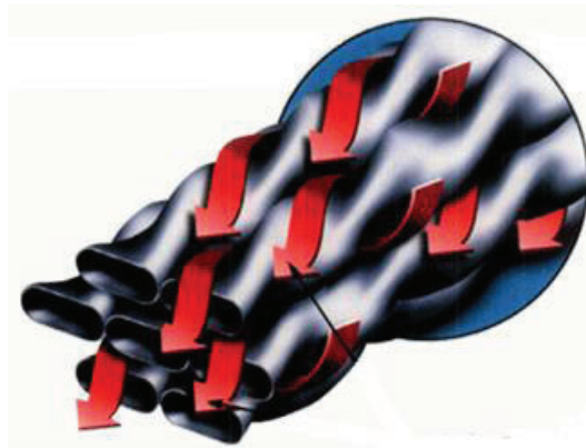
Figure 5. Twisted heat exchanger tubes at UNM [12].
