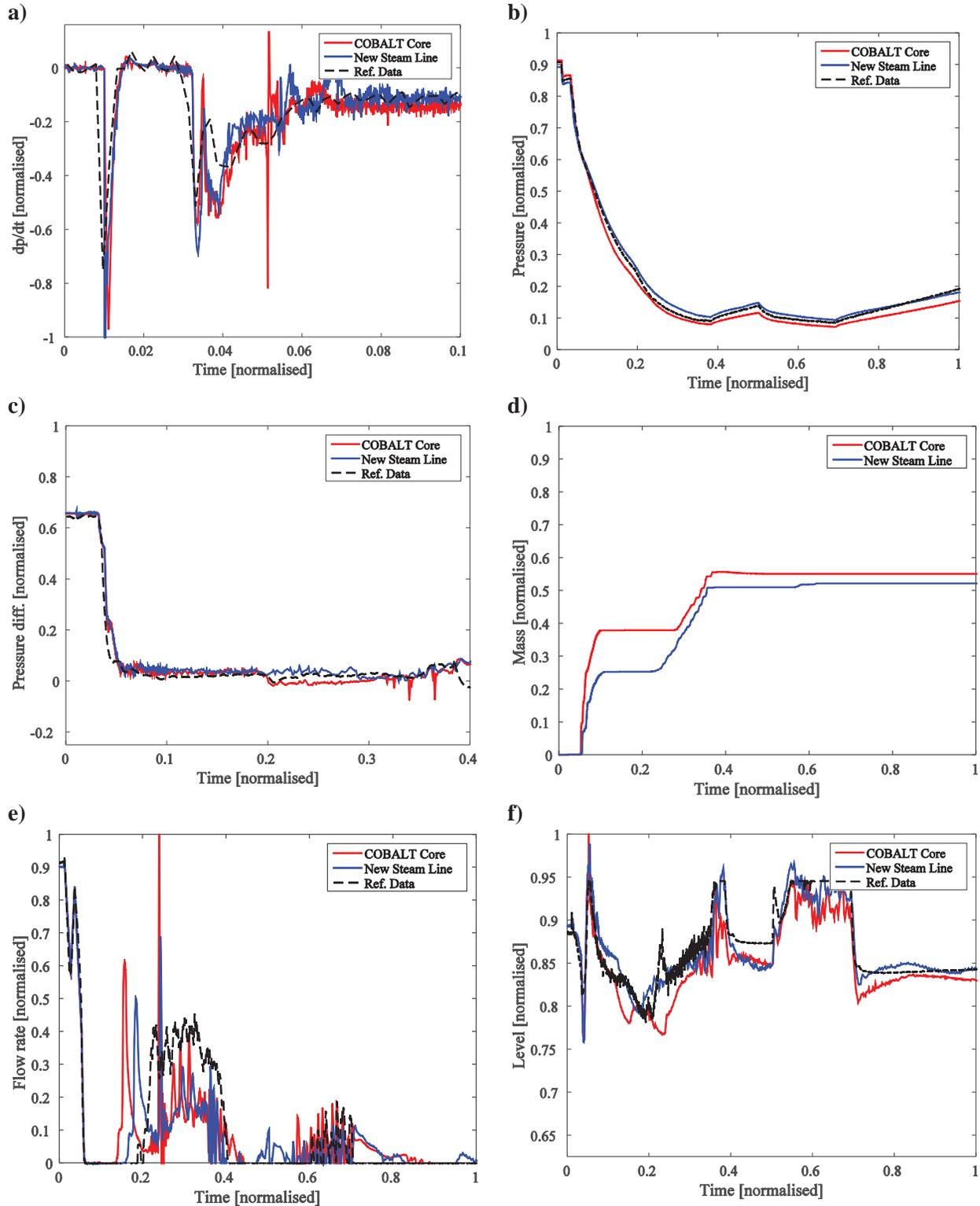
**Figure 7. ADS QoIs for “COBALT Core” and “New Steam Line” models: a) Dome pressure time derivative  $dp/dt$  (detail beginning of transient), b) RPV dome pressure, c)  $\Delta P$  core lower support plate (detail beginning of transient), d) Steam line water carry-over, e) Mass flow through the feed-water line and f) Wide range core level.**
