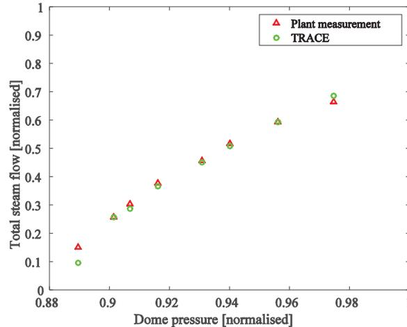
**Figure 6. Steam line stand alone model: verification of total steam flow vs. plant data for different rated and off rated plant conditions (dome pressures).**
