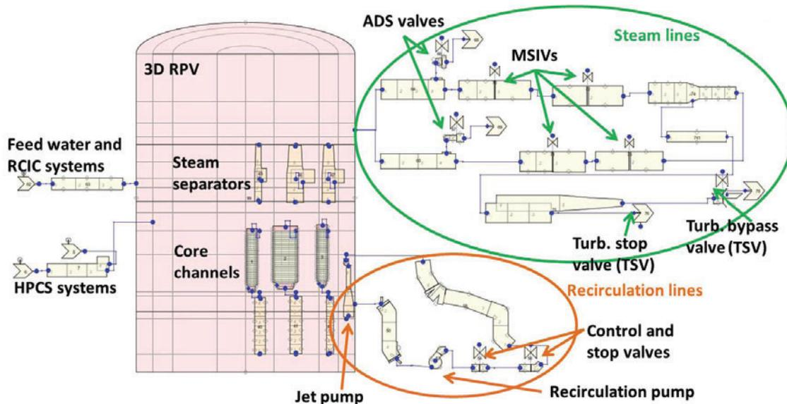
Figure 2. TRACE initial nodalisation of BWR/6 plant.
