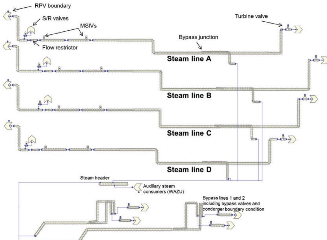
Figure 5. Steam lines with their bypasses. New TRACE nodalisation scheme.
