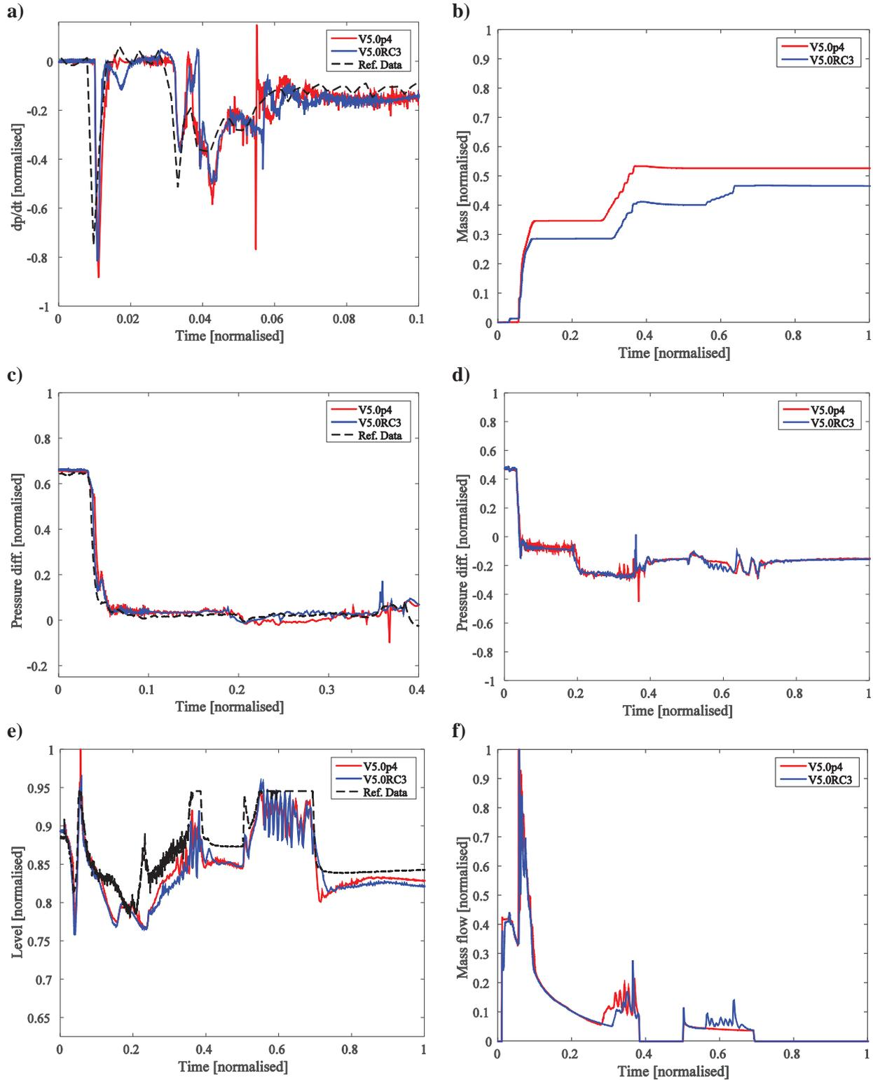
**Figure 3. ADS QoIs for different code versions: a) Dome pressure time derivative  $dp/dt$  (detail beginning of transient), b) Steam line water carry-over, c)  $\Delta P$  core lower support plate (detail beginning of transient), d)  $\Delta P$  channel wall, e) Wide range core level and f) Mass flow through the ADS valves.**
