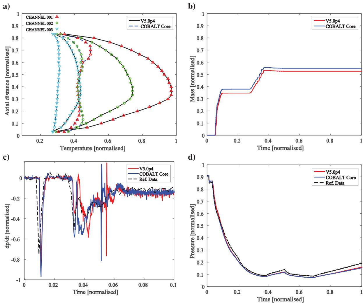
Figure 4. ADS QoIs for the TRACEv5.0p4 and the ‘COBALT Core’ models: a) Initial axial fuel temperature distribution, b) Steam line water carry-over, c) Dome pressure time derivative  $dp/dt$  (detail beginning of transient) and d) RPV dome pressure.
