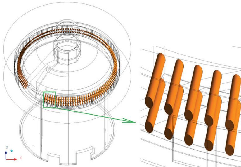
Figure 8. CFX Model – Air Inlet Details
