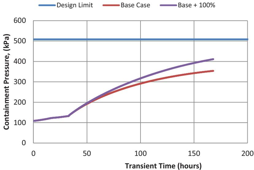
Figure 4. Containment Pressure – Loss of Shutdown Cooling during Refueling (4 MW of decay heat within containment)
