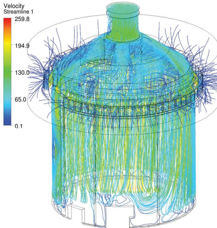
Figure 13. AP1000® Full-Scale PCS Air Flow Model – Streamlines
