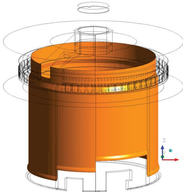
Figure 9. CFX Model – Air Baffle Details
