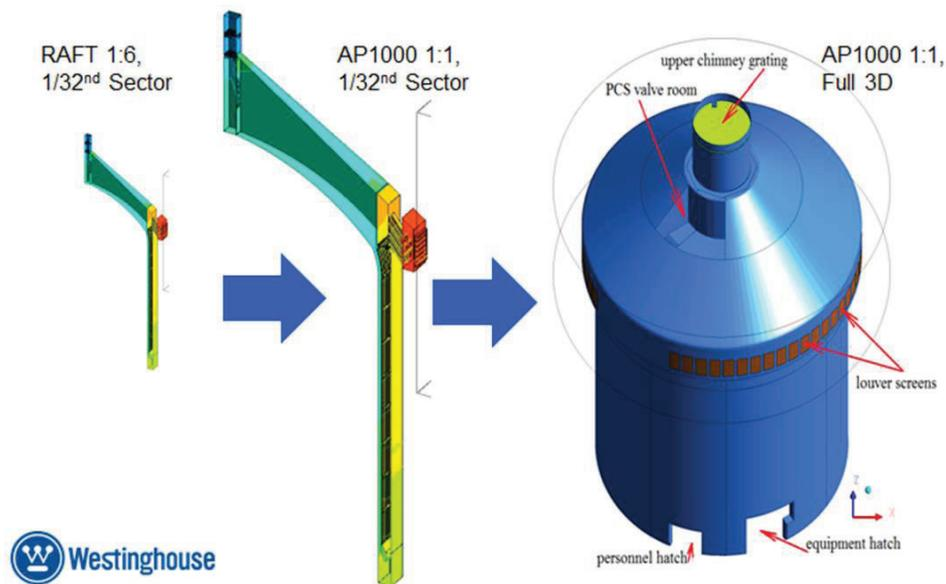
Figure 7. CFD Model Evolution from RAFT to Full-Scale, 3D AP1000®
