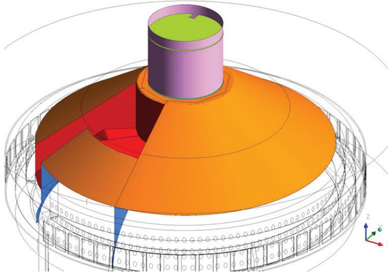
Figure 10. CFX Model Air Outlet Details
