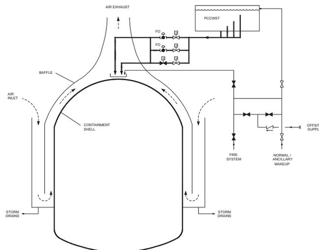
Figure 1. AP1000® Passive Containment Cooling System
