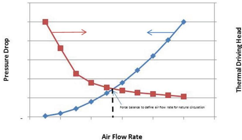
Figure 2. Natural Circulation Flow Force Balance
