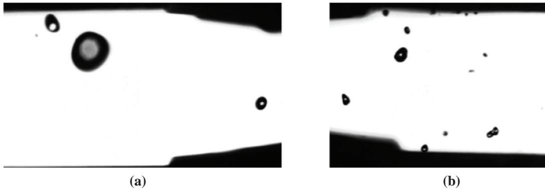
Figure 9. Examples of Droplet images near the Blockage Region for 90% short blockage. (a: upstream, b: downstream)
