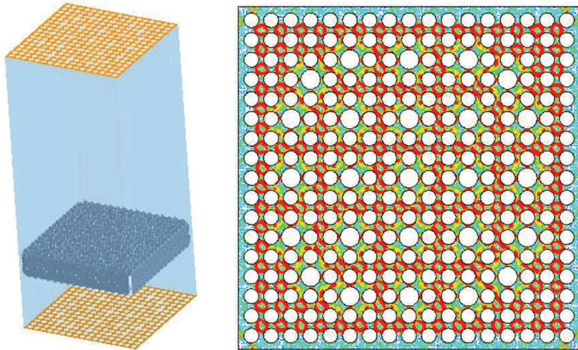
**Figure 8. Model geometry and flow field for a typical single-span 17x17 spacer grid simulation.**
