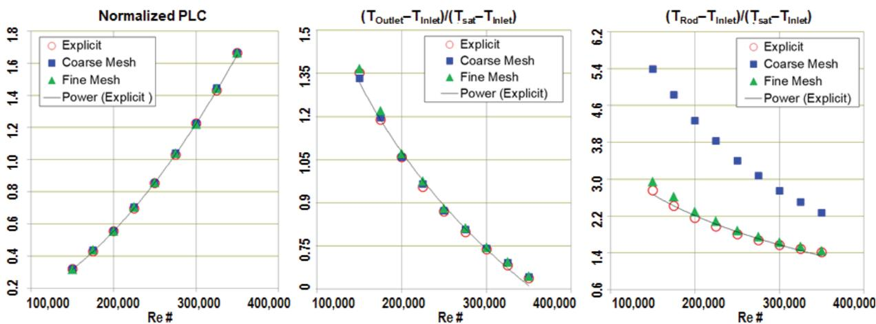
Figure 11. Source-based sub-channel average predictions dependence on mesh refinement.
