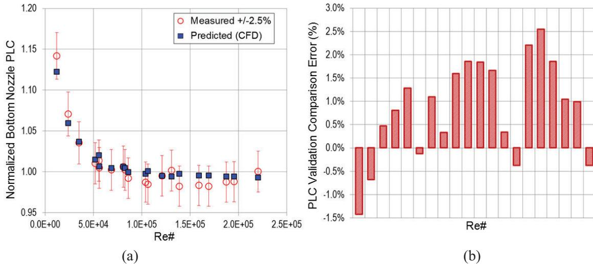
Figure 6. Validation of Bottom Nozzle PLC prediction method.
