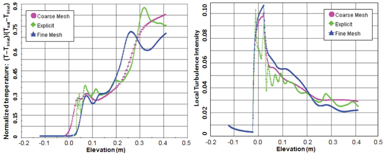
Figure 10. Source-based local predictions dependence on mesh refinement.
