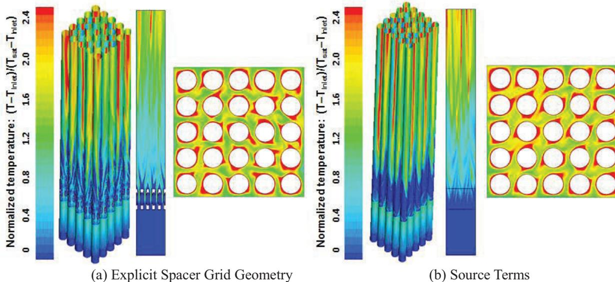
Figure 9. Calibration of source-based modeling of spacer grids against explicit geometry.
