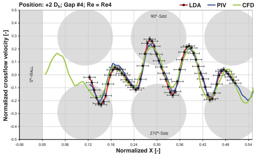
Figure 5. Comparison between the measured and predicted cross-flow velocity profiles 2 Dh downstream of the spacer grid.
