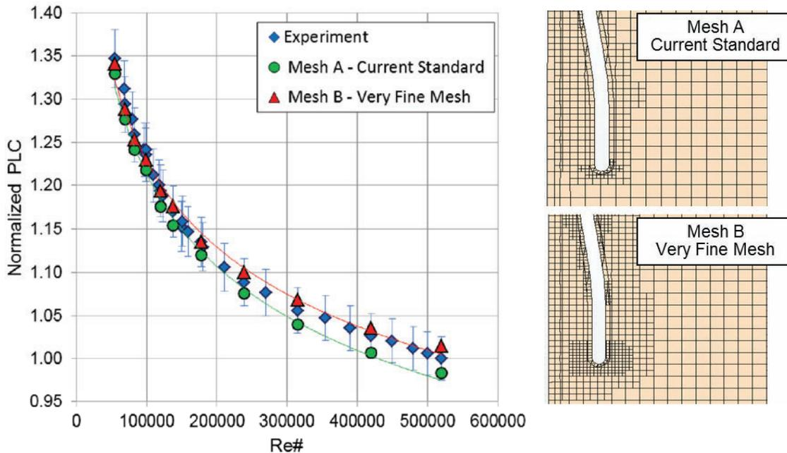
**Figure 3. Mesh Refinement impact on prediction accuracy on a 17x17 mixing vane spacer model for PLC predictions in support of product licensing.**
