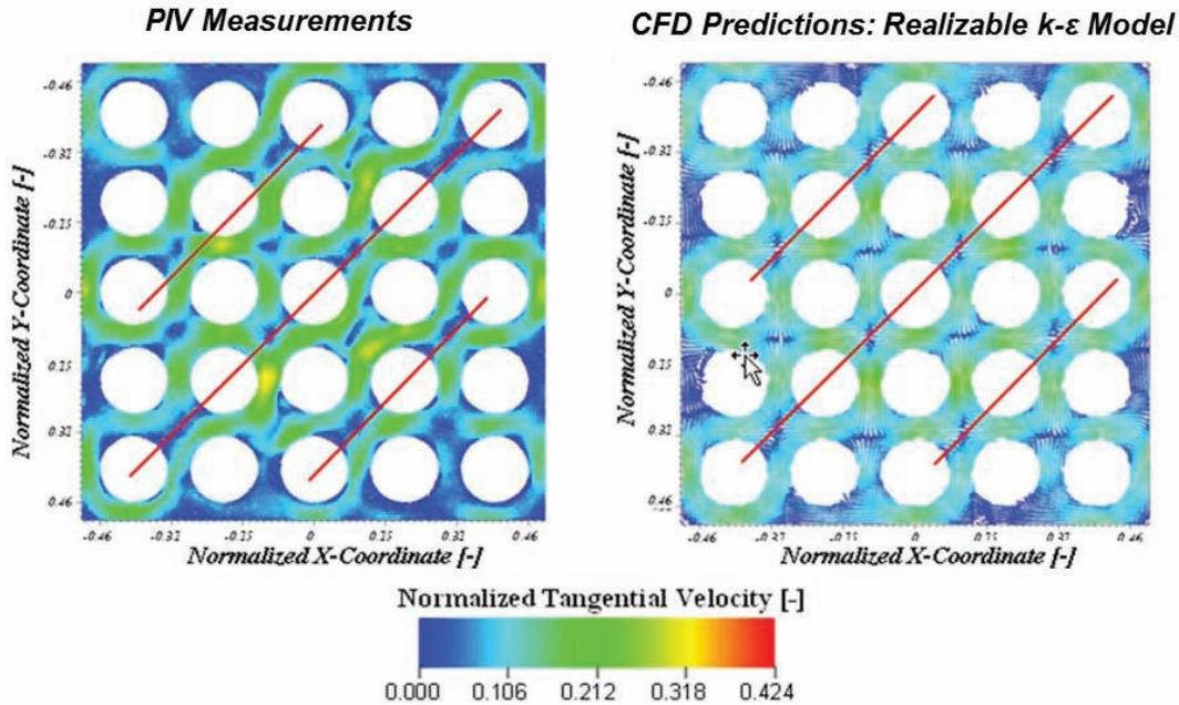
Figure 4. Comparison between the measured and predicted velocity profiles 8 Dh downstream of the spacer grid.
