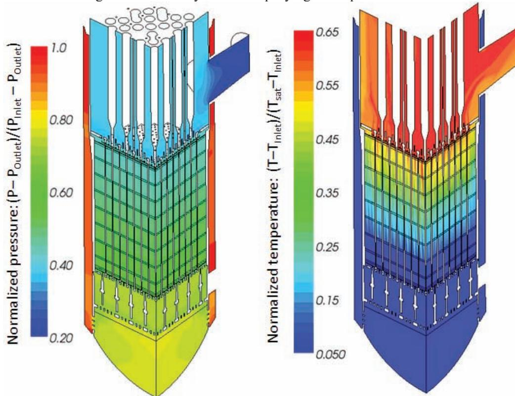
**Figure 12. Source-based quarter reactor core thermal analysis.**
