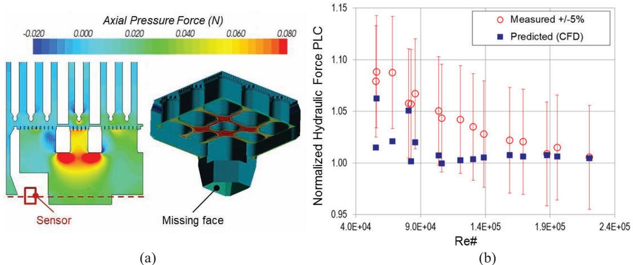
Figure 7. Validation of CFD methodology for Hydraulic Force prediction.
