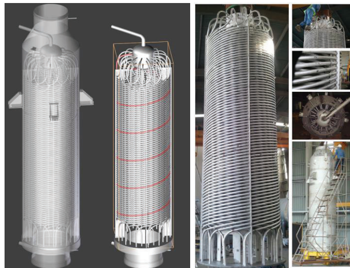
Figure 2. Sodium-to-air heat exchanger (AHX) of STELLA-1
