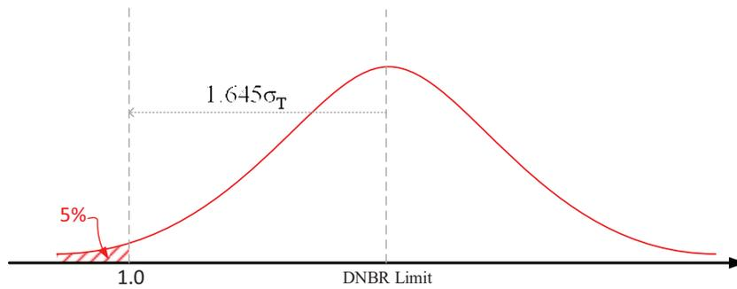
Figure 5. Schematic Diagram for Determining the DNBR Limit
