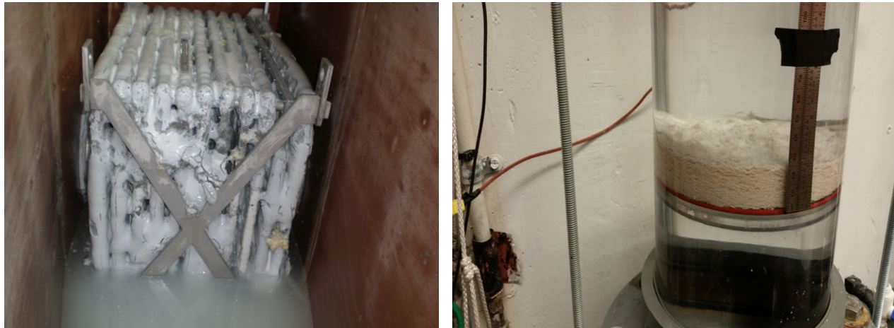
Figure 1. Debris accumulation on sump strainer module for previous tests [15] (left) and UNM vertical head loss column tests [7-10]
