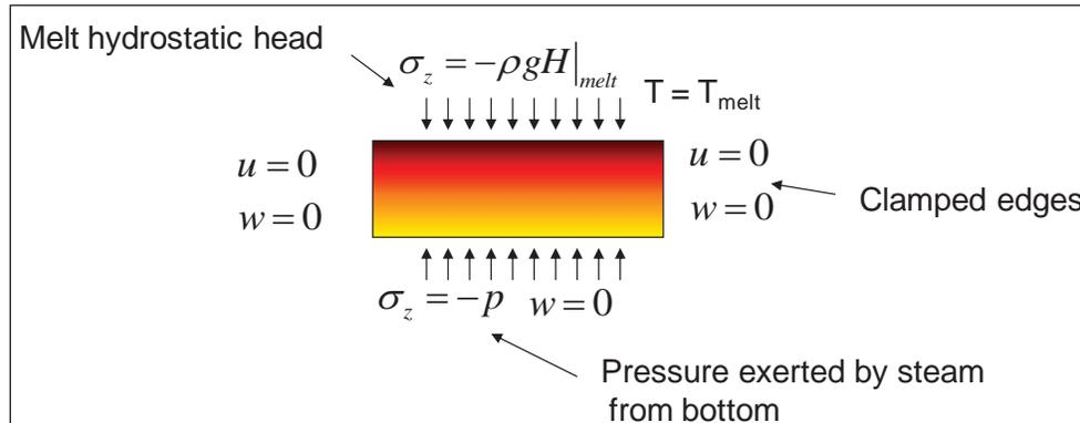
**Figure 5: Stresses in the crust.**
