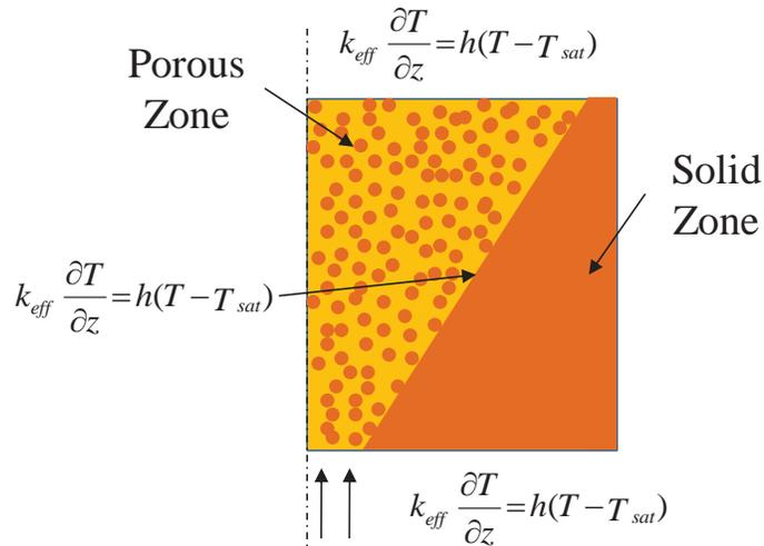
**Figure 7: Modified boundary conditions for the domain**
