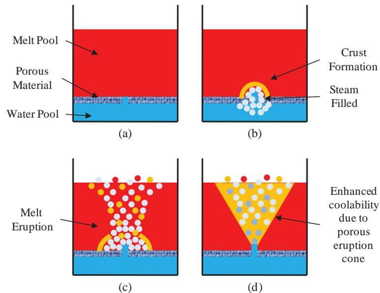
**Figure 1: Melt coolability under bottom flooding with decay heat model**
