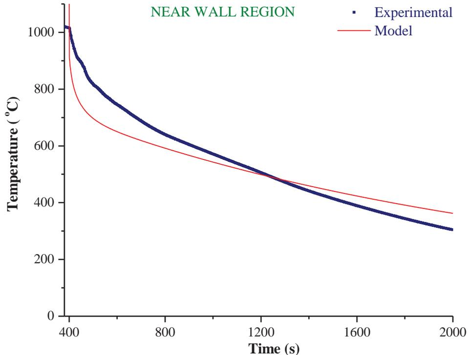
**Figure 10: Modeled vis-à-vis measured temperatures near inner wall of the test section**
