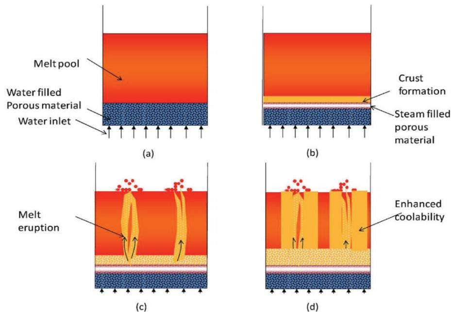
Figure 2: Melt coolability model by Kulkarni and Nayak (2013)
