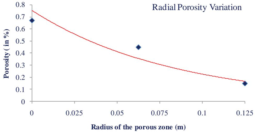
Figure 3: Variation in porosity along the radius of the porous zone within the test section
