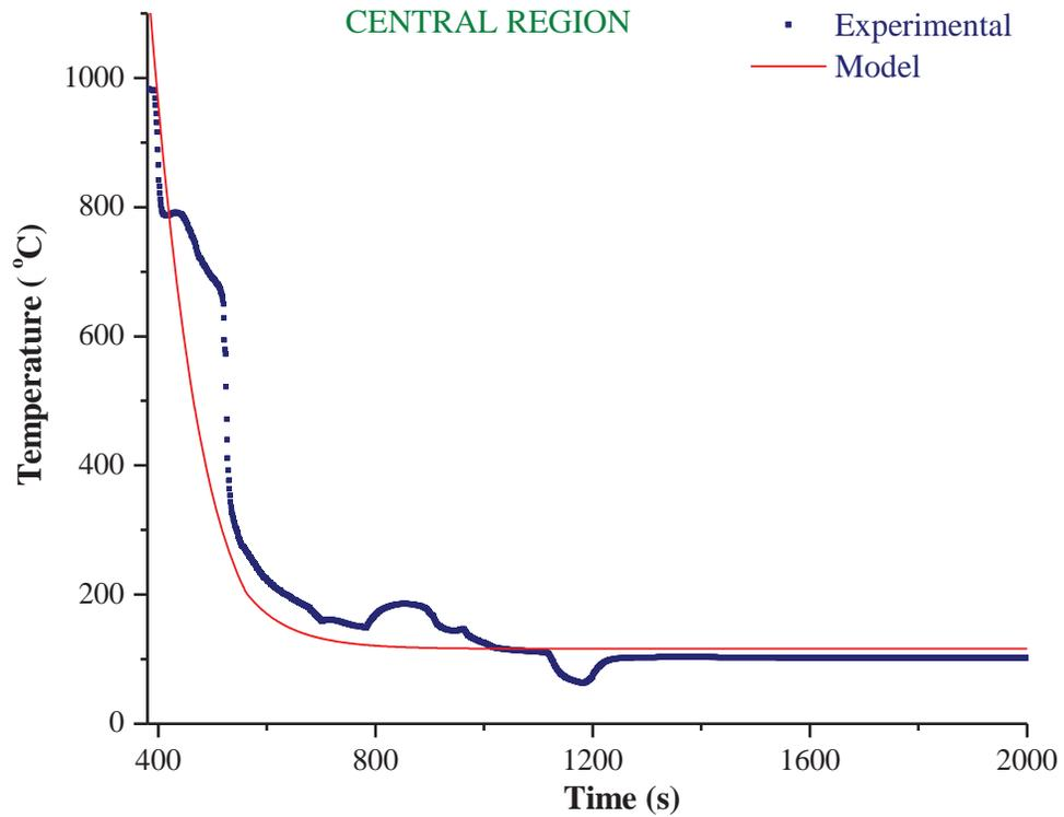
**Figure 8: Modeled vis-à-vis measured temperatures at central location of the test section**
