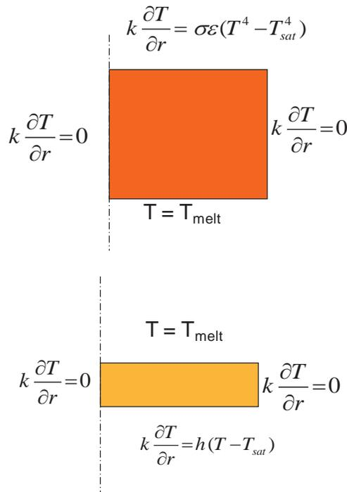
Figure 4: Boundary conditions for melt and crust layer.
