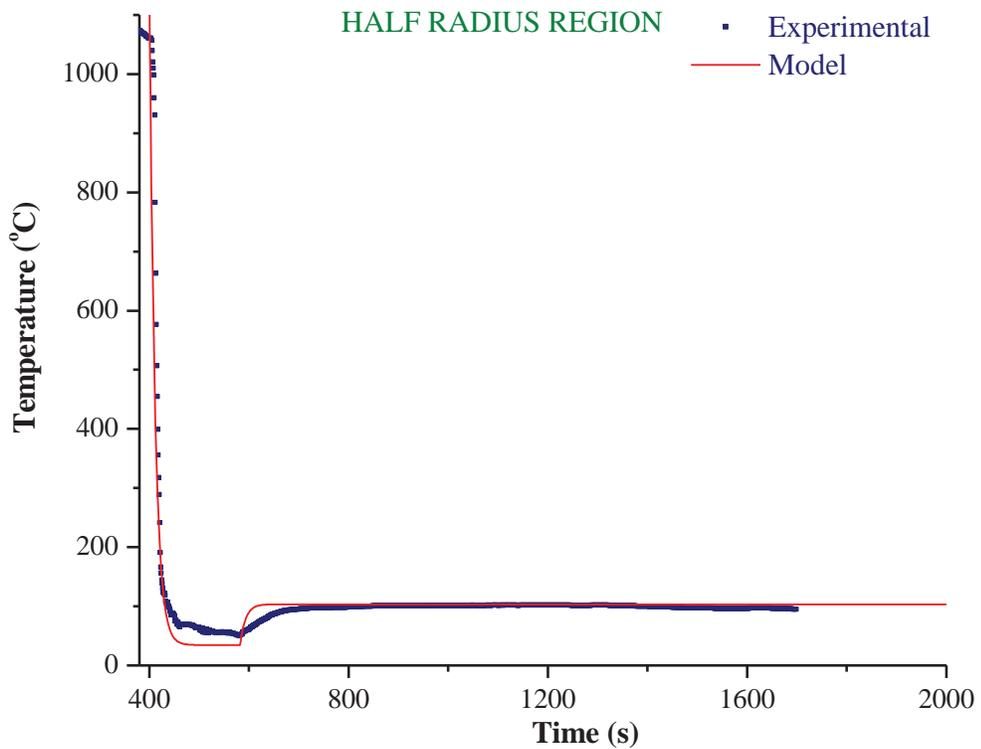
**Figure 9: Modeled vis-à-vis measured temperatures at Half Radius of the test section**
