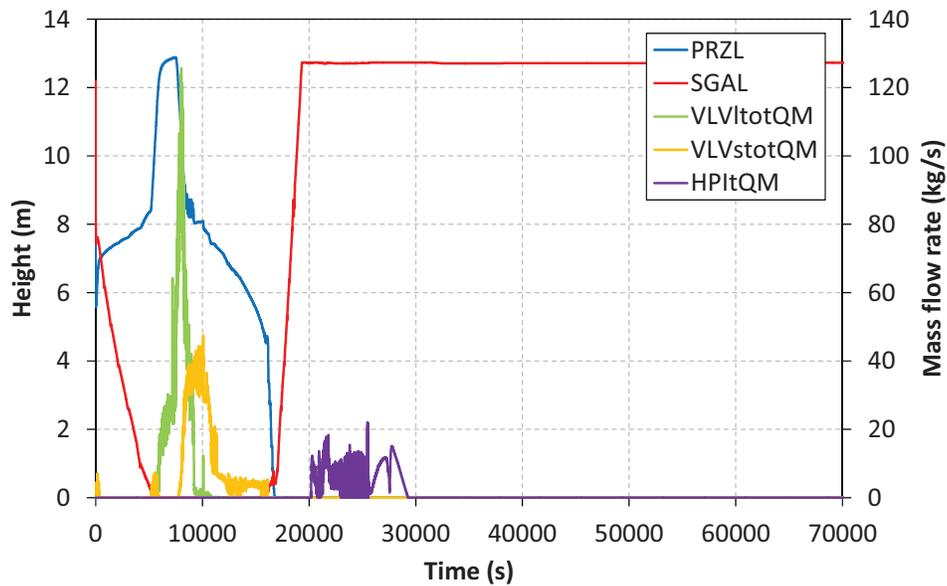
**Figure 6 Pressurizer and Steam Generator Level and Mass Flow Rates through Pressurizer Valves and HPI**
