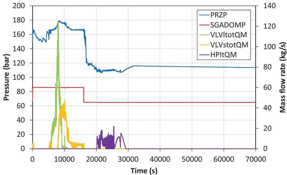
Figure 5 System Pressures and Mass Flow Rates through Pressurizer Valves and HPI
