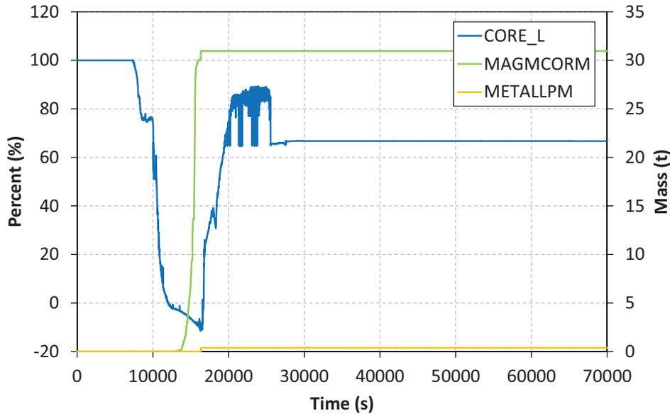
**Figure 7 Percentage of Core Water Level and degraded Core Materials**
