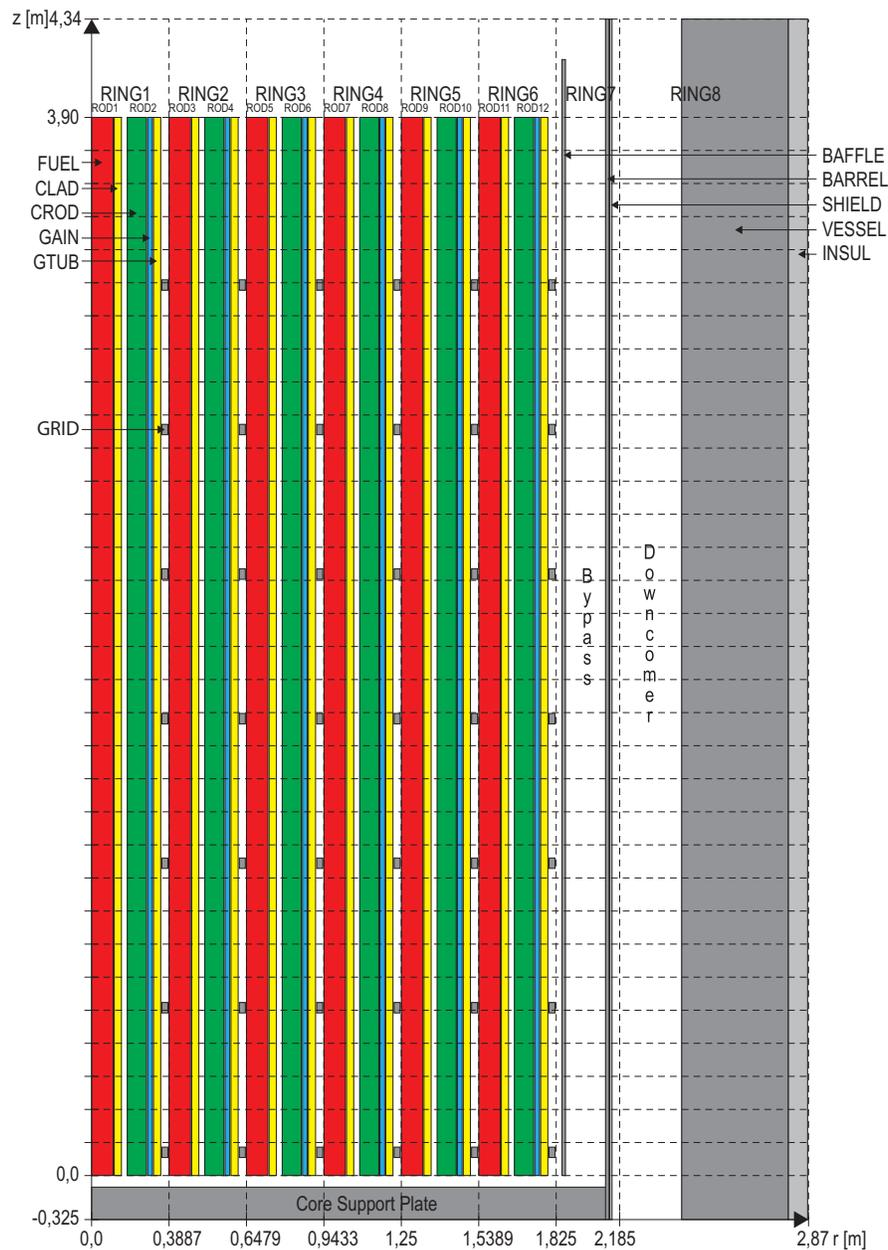
Figure 3 Reactor Core Modelling in ASTEC
