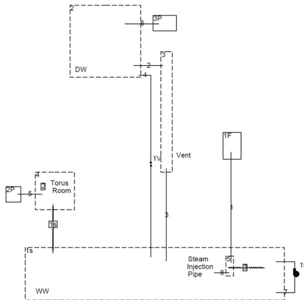
**Figure 6: GOTHIC BFN Unit 2 Lumped Model Nodalization**
