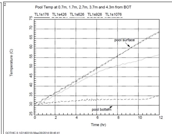
**Figure 3: Suppression Pool Temperature**
