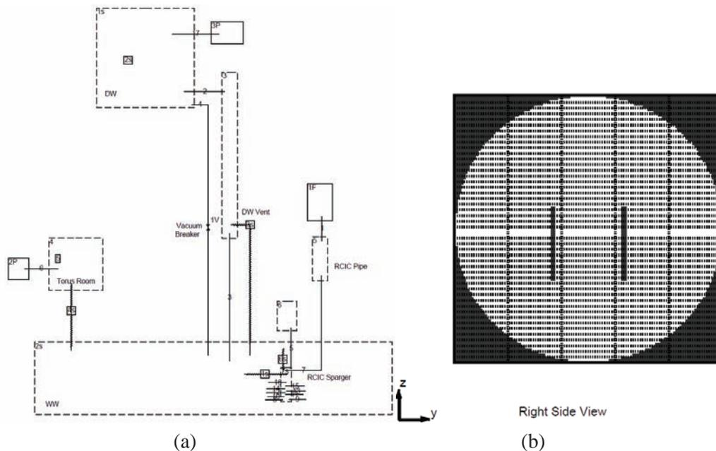
**Figure 1: GOTHIC BFN 3D Model Nodalization (a) and Suppression Pool Mesh (b)**
