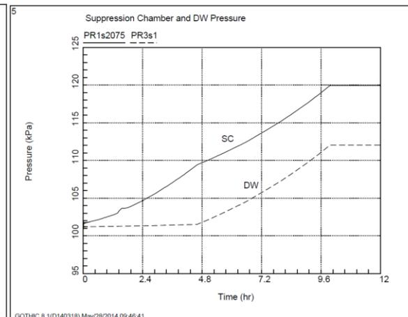
**Figure 5: Torus and Drywell Pressure**
