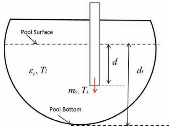
**Figure 7: Suppression Pool Parameters**
