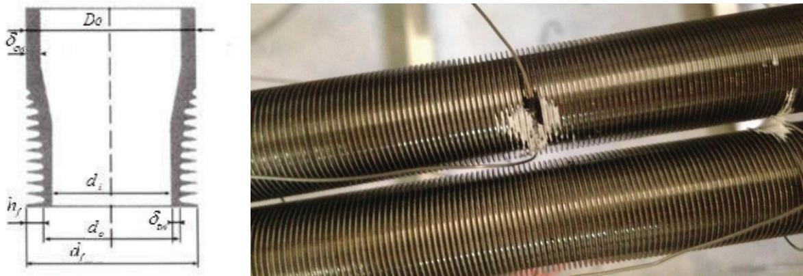
**Figure 1.2. Fined-tube of the Reheater.**
