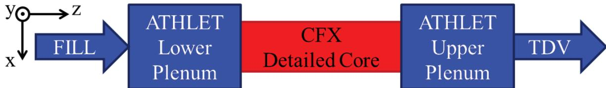
Figure 4. Simple setup for testing of the CFX/ATHLET-coupling.
