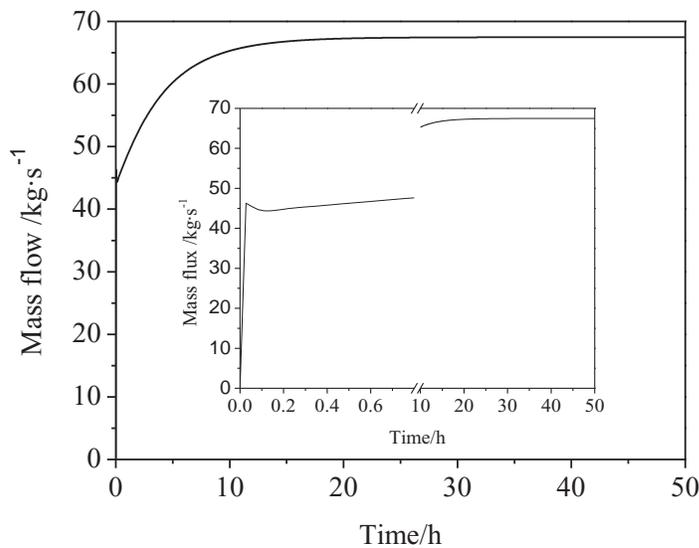
Fig. 7 The coolant mass flux change of the passive cooling system
