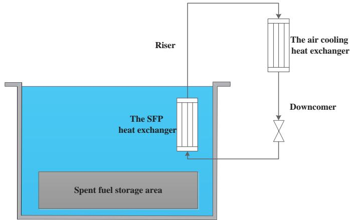
Fig. 1 Design diagram of passive cooling system
