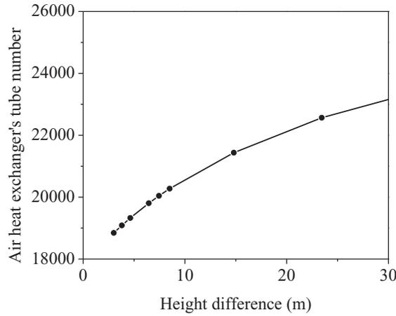
Fig. 3 The curve of tube number of the air heat exchanger with height difference
