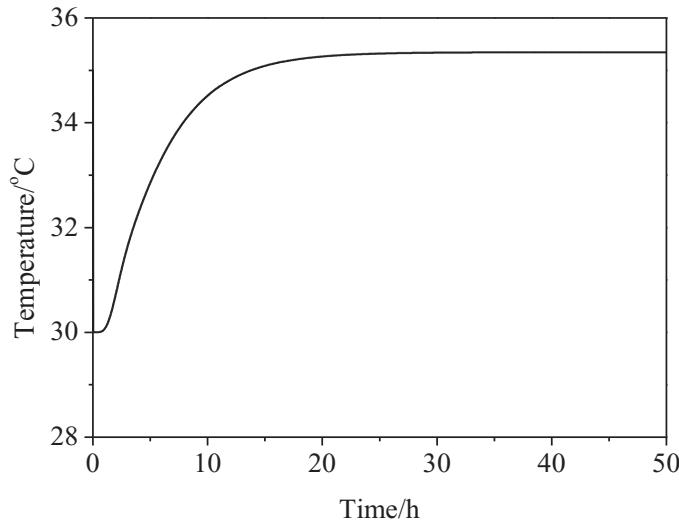
Fig. 10 The inlet temperature of the SFP heat exchanger
