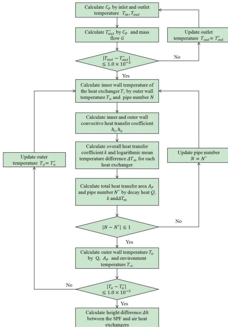
Fig. 2 Calculation flow chart of the passive cooling system
