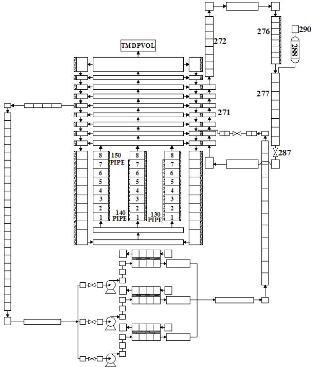
Fig. 6 Nodalization of the passive cooling system
