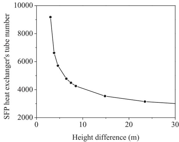
Fig. 4 The curve of tube number of the SFP heat exchanger with height difference
