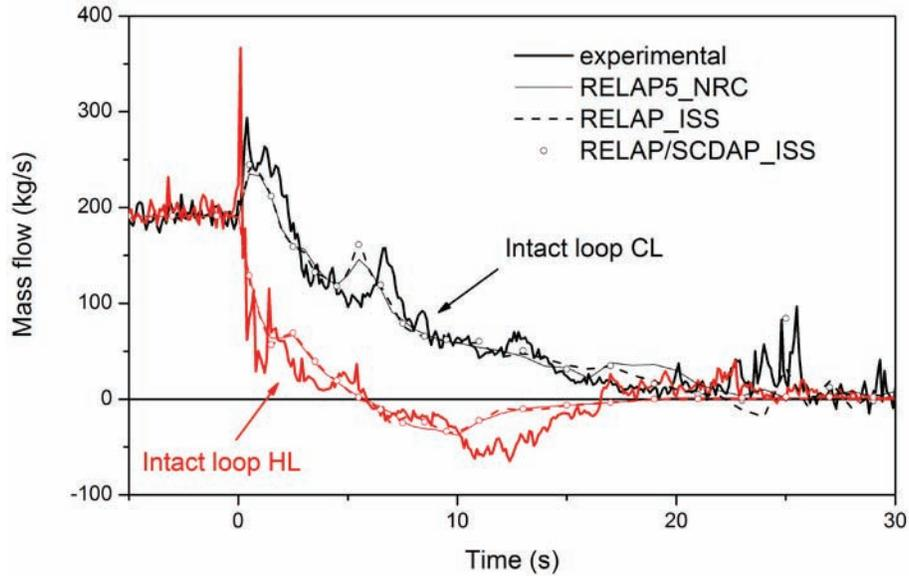
**Figure 5 Intact loop HL and CL mass flows**
