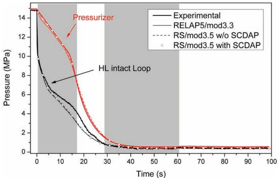
**Figure 4 Intact loop HL and Pressurizer pressures**
