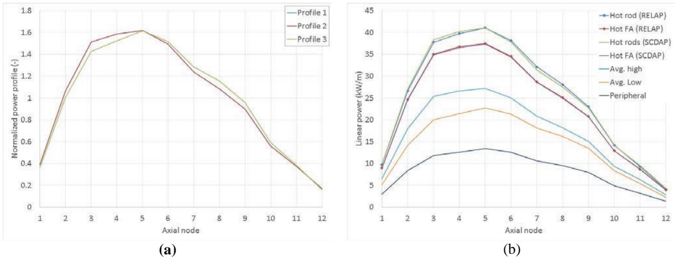
**Figure 2. (a) Power profiles; and (b) Linear power per each fuel rod type**
