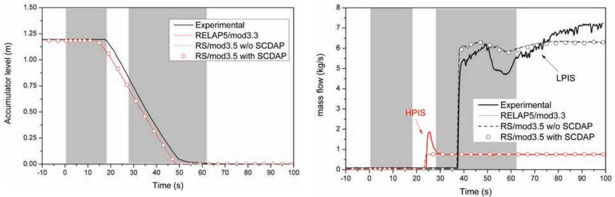
**Figure 8 Left: Accumulator level. Right: HPIS and LPIS mass flows**
