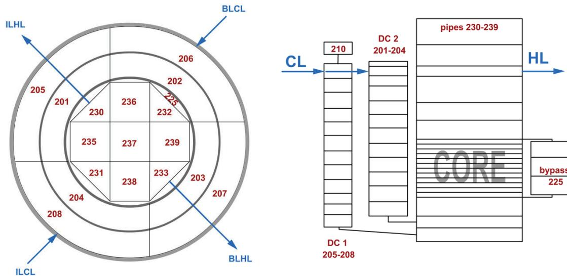
**Figure 1. Scheme of the nodalization of the Reactor Pressure Vessel for the LOFT facility (left: top view, right: axial view)**
