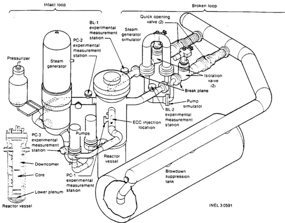
Figure 3 LOFT system configuration for cold leg break
