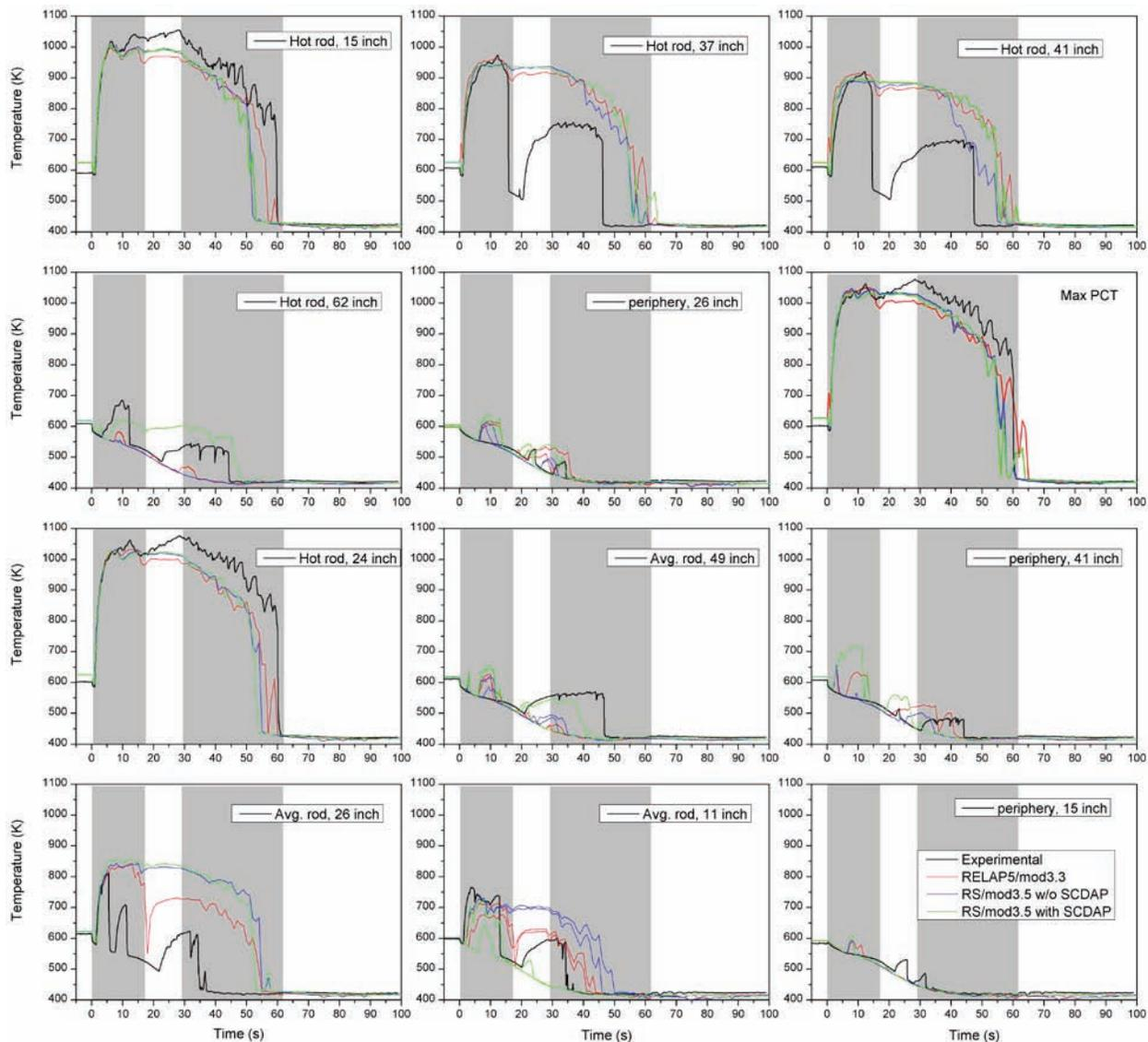
**Figure 9 Cladding temperatures in different parts of the core.**
