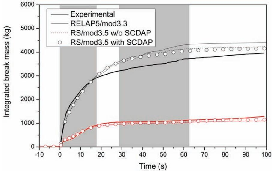
**Figure 7 Integrated discharged mass**
