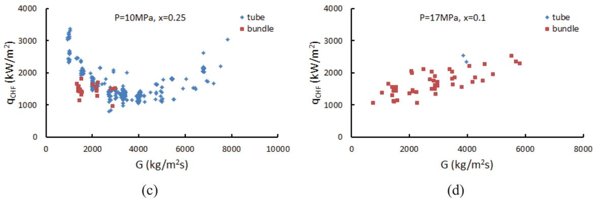
Figure 8. Comparison of CHF Trend in Tube and Bundle with Mass Flux
