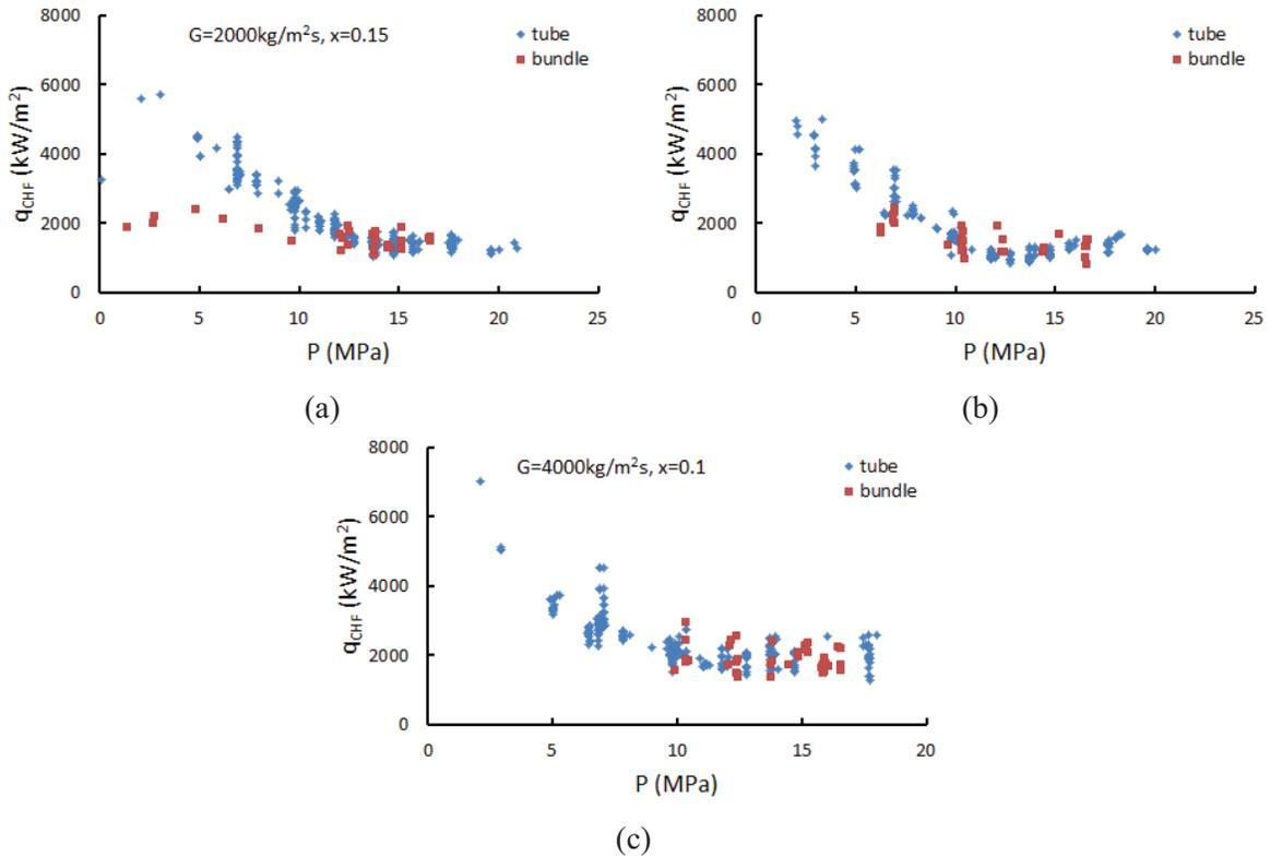
Figure 7. Comparison of CHF Trend in Tube and Bundle with Pressure
