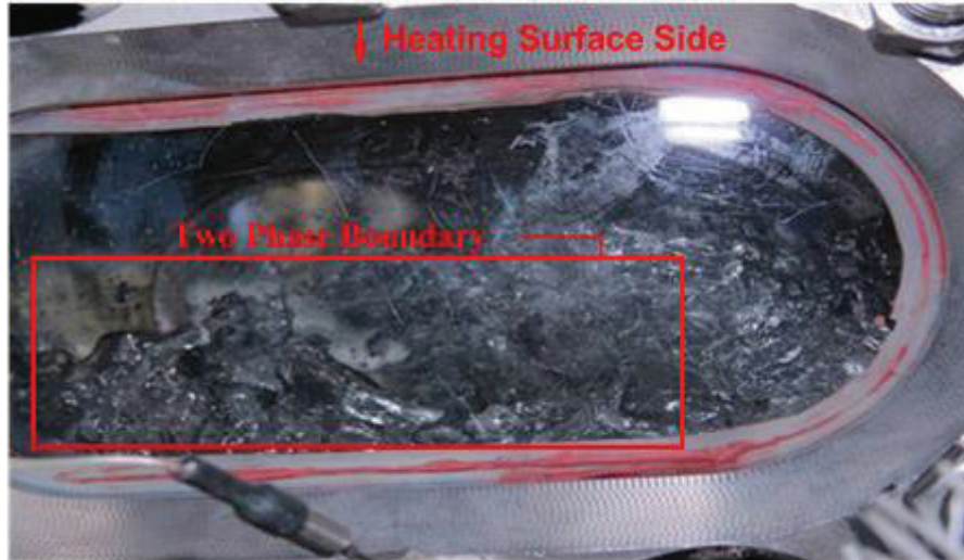
Figure 4. Visualization of Bubble Behavior in the Chamber
