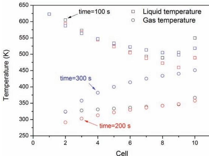
**Figure 10 Gas and liquid temperature profiles across the test section for the vertical set-up**
