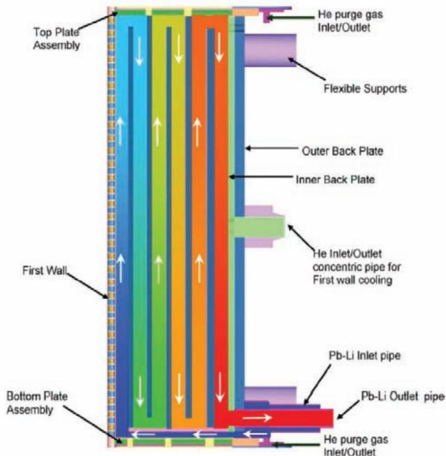
**Figure 1 Schematic of LLCB blanket concept [1]**
