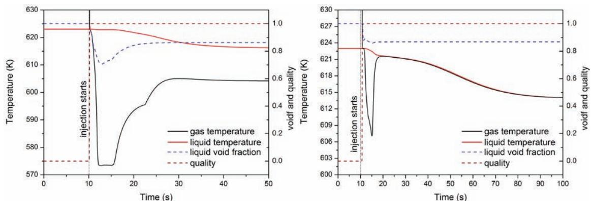
**Figure 5 Fluid temperatures, quality and liquid void fraction for the horizontal set-up at the injection point (left) and at the test section exit (right)**
