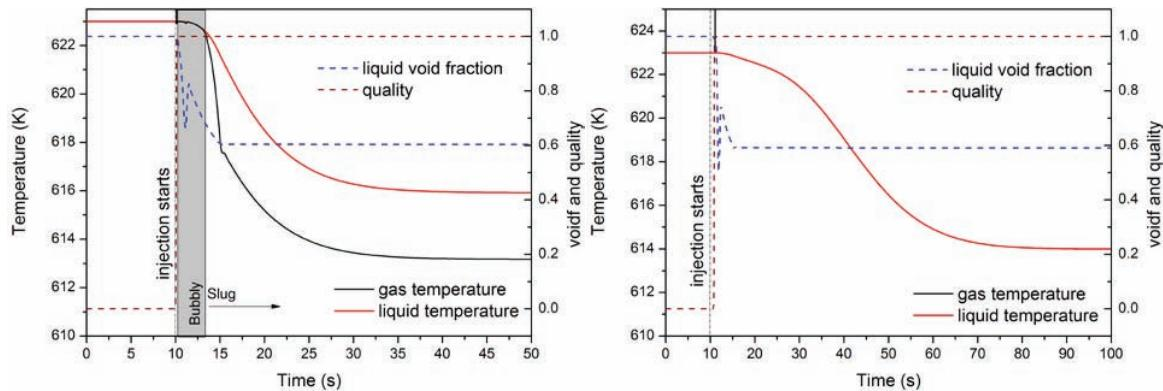
**Figure 3 Fluid temperatures, quality and liquid void fraction for the vertical set-up at the injection point (left) and at the test section exit (right)**
