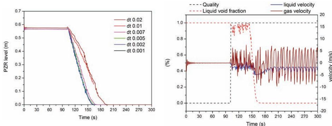
**Figure 6 Horizontal set-up including a PZR. PZR collapsed water level (left). Quality and liquid void fraction at the bottom of the PZR**
