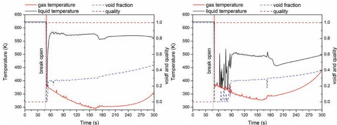
**Figure 9 Fluid temperatures, quality and liquid void fraction for the vertical set-up with break at the break connection (left) and at the test section exit (right)**
