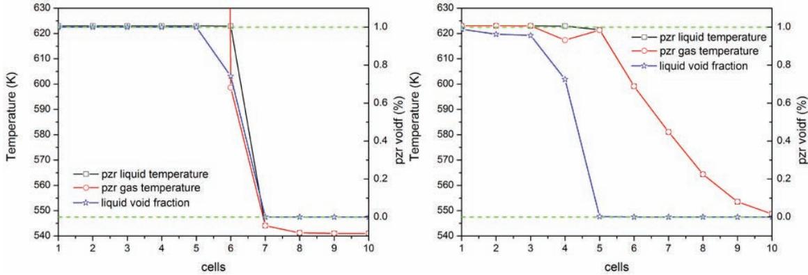
**Figure 7 Profiles for liquid void fraction and fluid temperatures across the PZR for the horizontal set-up including a PZR at time=90s (left) and time=120s (right)**
