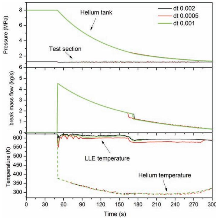
**Figure 8 Results for the break set-up with different time steps. Top graph: helium tank and test section pressures. Mid graph: break mass flow. Bottom graph: LLE and He temperatures in the test section, cell 2**
