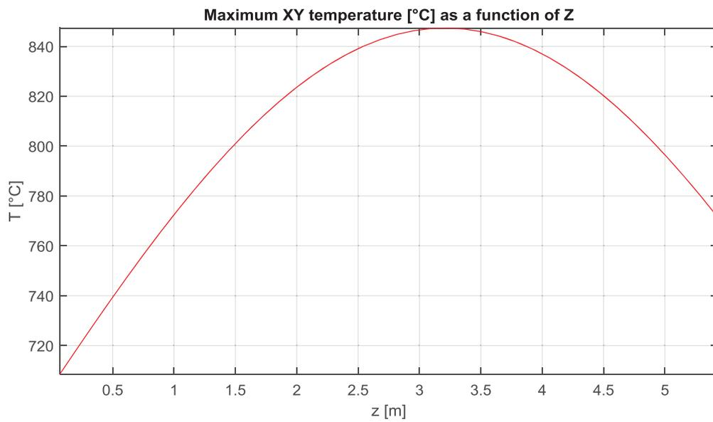
Figure 10. Axial distribution of the maximum fuel temperature
