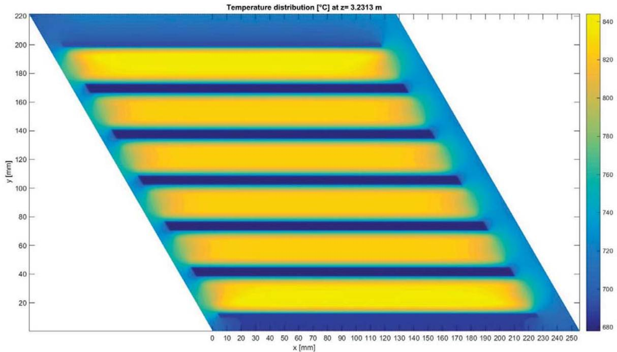
**Figure 11. XY temperature distribution at the location of the maximum**
