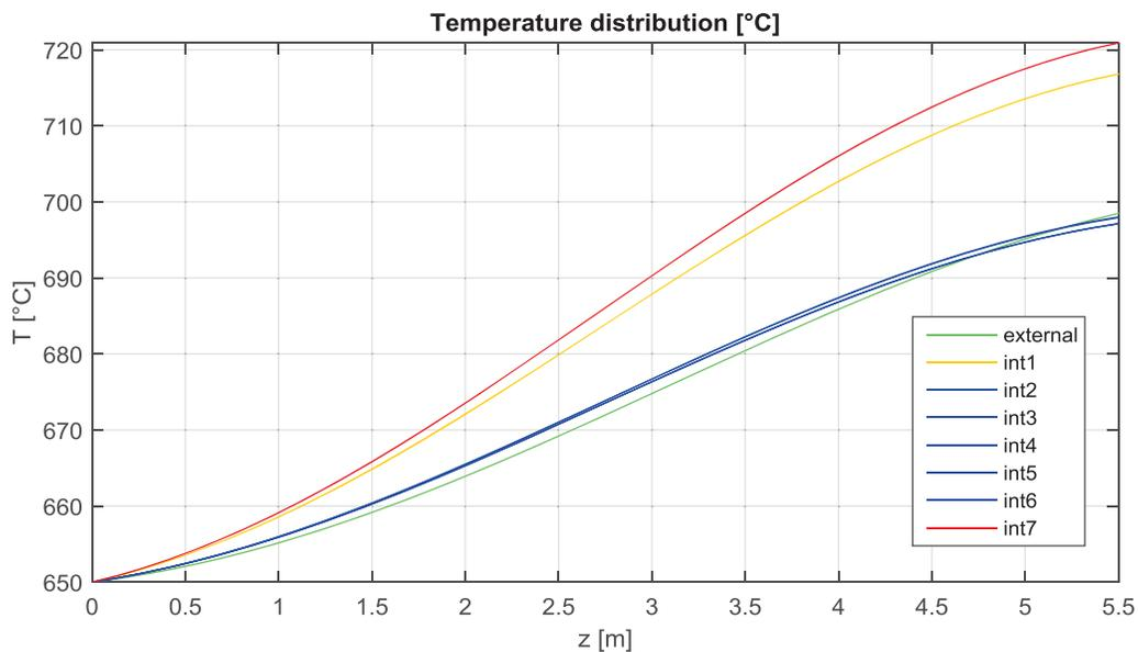
**Figure 12. Axial temperature distribution of the channels**
