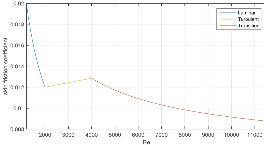
**Figure 4. Skin friction coefficient as a function of Re**
