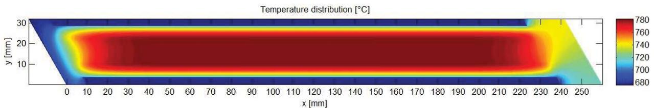
**Figure 8. Temperature distribution of the single plate (1630x400 nodes)**
