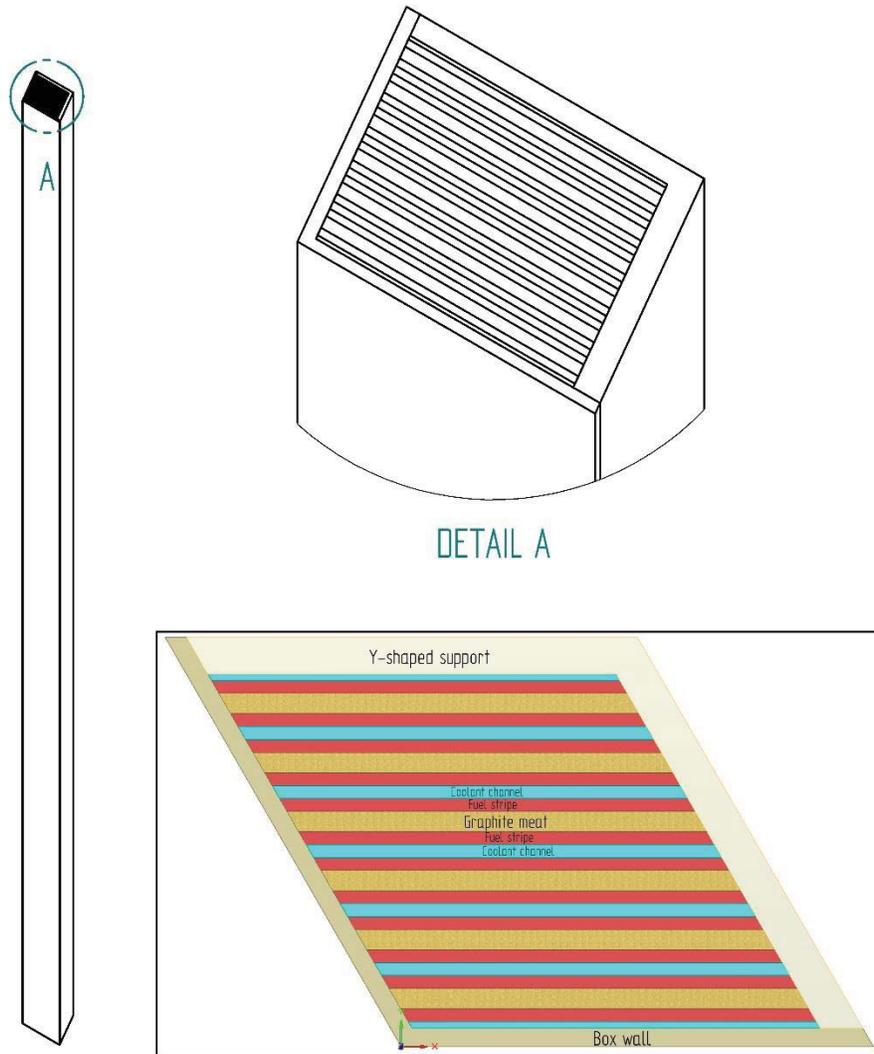
**Figure 1. Details of the fuel assembly model**
