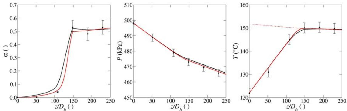
**Figure 3. Comparison of baseline results (black) and original RELAP5 subcooled boiling model (red) at intermediate pressure and low flow conditions: a) void fraction, b) pressure, c) liquid (solid) and saturation (dashed) temperatures. Conditions:  $P_{in} = 498$  kPa,  $j_{f,in} = 0.24$  m/s,  $\Delta T_{sub,in} = 30^\circ\text{C}$ ,  $q_w'' = 156$  kW/m<sup>2</sup>.**
