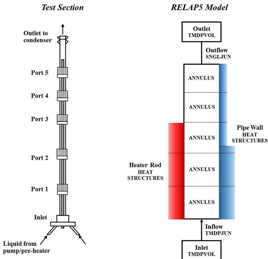
Figure 1. Sketch of the experimental test section (left) and RELAP5 nodalization (right).
