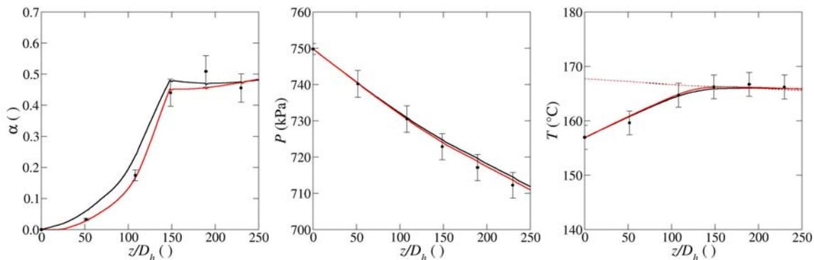
**Figure 2. Comparison of baseline results (black) and original RELAP5 subcooled boiling model (red) at elevated pressure and high flow conditions: a) void fraction, b) pressure, c) liquid (solid) and saturation (dashed) temperatures. Conditions:  $P_{in} = 750$  kPa,  $j_{f,in} = 1.0$  m/s,  $\Delta T_{sub,in} = 11^\circ\text{C}$ ,  $q_w'' = 241$  kW/m<sup>2</sup>.**
