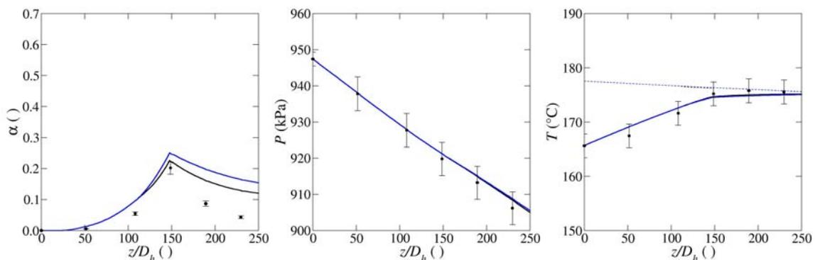
**Figure 5. Comparison of baseline results (black) and the new condensation model (blue): a) void fraction, b) pressure, c) liquid (solid) and saturation (dashed) temperatures. Conditions:  $P_{in} = 947$  kPa,  $j_{f,in} = 1.0$  m/s,  $\Delta T_{sub,in} = 12^\circ\text{C}$ ,  $q_w'' = 209$  kW/m<sup>2</sup>.**
