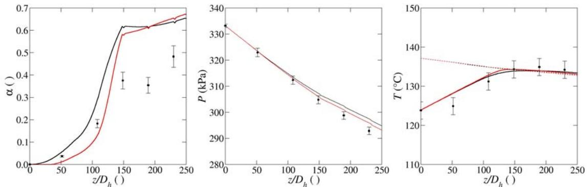
**Figure 4. Comparison of baseline results (black) and original RELAP5 subcooled boiling model (red) at low pressure and high flow conditions: a) void fraction, b) pressure, c) liquid (solid) and saturation (dashed) temperatures. Conditions:  $P_{in} = 333$  kPa,  $j_{f,in} = 1.0$  m/s,  $\Delta T_{sub,in} = 13^\circ\text{C}$ ,  $q_w'' = 264$  kW/m<sup>2</sup>.**
