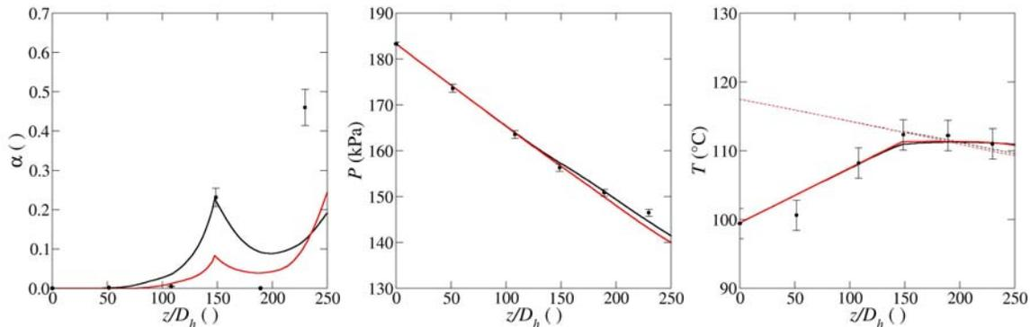
**Figure 7. Comparison of baseline results (black) and original RELAP5 subcooled boiling model (red): a) void fraction, b) pressure, c) liquid (solid) and saturation (dashed) temperatures. Conditions:  $P_{in} = 183$  kPa,  $j_{f,in} = 0.24$  m/s,  $\Delta T_{sub,in} = 18^\circ\text{C}$ ,  $q_w'' = 61$  kW/m<sup>2</sup>.**
