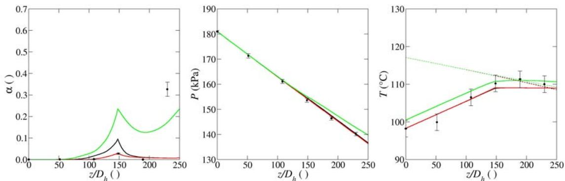
**Figure 6. Comparison of baseline results (black), original RELAP5 subcooled boiling model (red) and the baseline model with artificially high inlet temperature (green): a) void fraction, b) pressure, c) liquid (solid) and saturation (dashed) temperatures. Conditions:  $P_{in} = 181$  kPa,  $j_{f,in} = 0.24$  m/s,  $\Delta T_{sub,in} = 19^\circ\text{C}$ ,  $q_w'' = 56$  kW/m<sup>2</sup>.**
