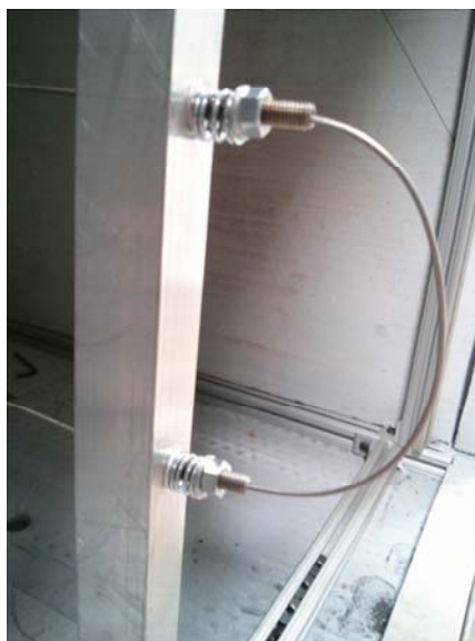
Figure 6: capillary in tension via springs and can be adjusted for changes over time
