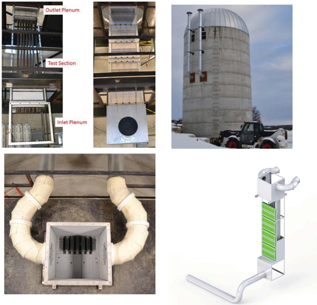
Figure 3: Top Left - as built view of the heated test section. Top Right - exterior of the ARCCS silo. Bottom Left - top view of the upper plenum. Bottom Right - solid works model of the entire system inside the silo.
