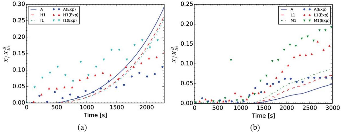
Figure 6. Helium molar fraction variations in Vessel-2, (a) ST3\_1, (b) ST3\_2.
