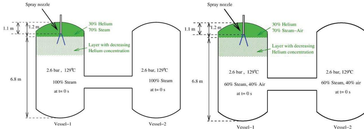
Figure 1. Initial conditions for the test (a) ST3\_1 and (b) ST3\_2 [6].
