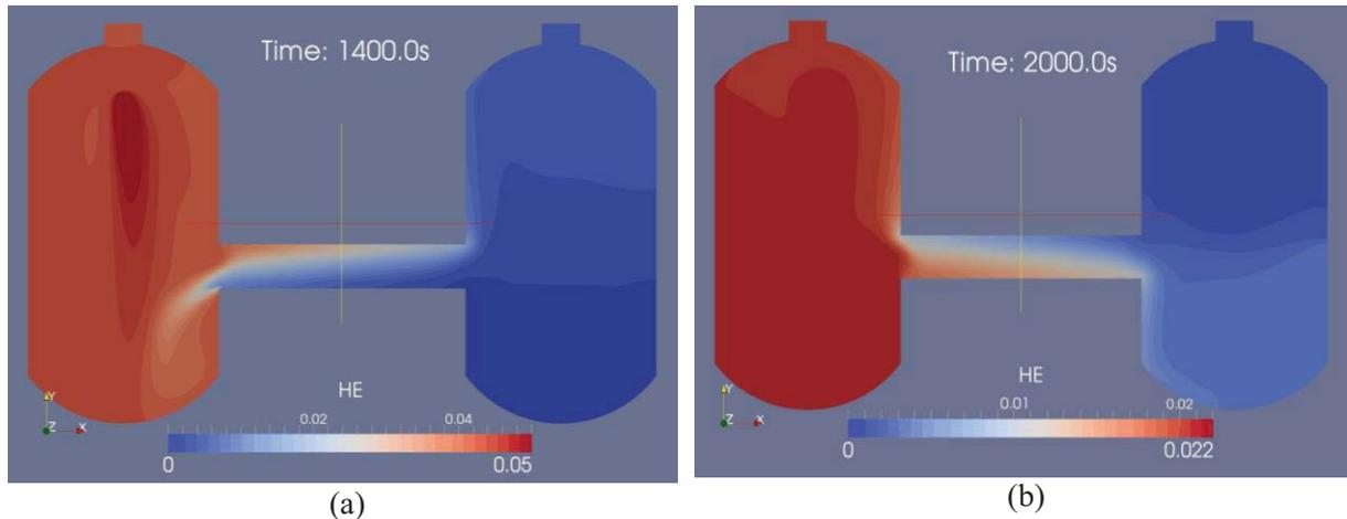
Figure 7. Helium mass fractions (a) ST3\_1, (b) ST3\_2.
