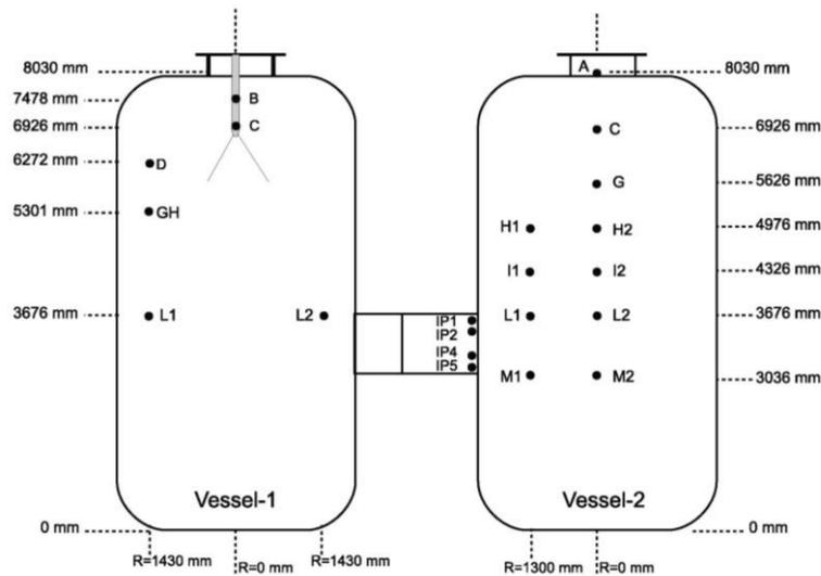
Figure 2. Gas concentration measurement locations in a vessel and interconnecting pipe (IP) [6].
