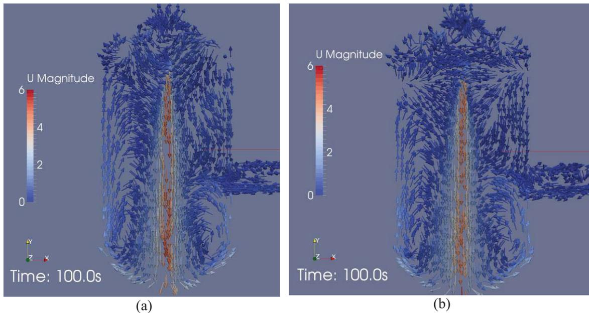
**Figure 5. Velocity vectors at  $t=100$  s in Vessel-1, (a) ST3\_1, (b) ST3\_2. Velocity magnitude unit is m/s.**
