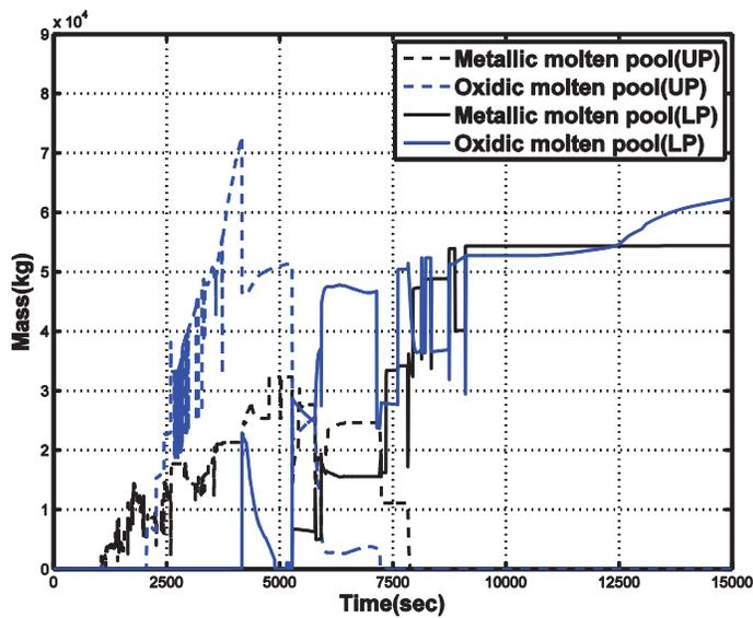
Figure 11. Mass of molten pools in the upper and lower plenum
