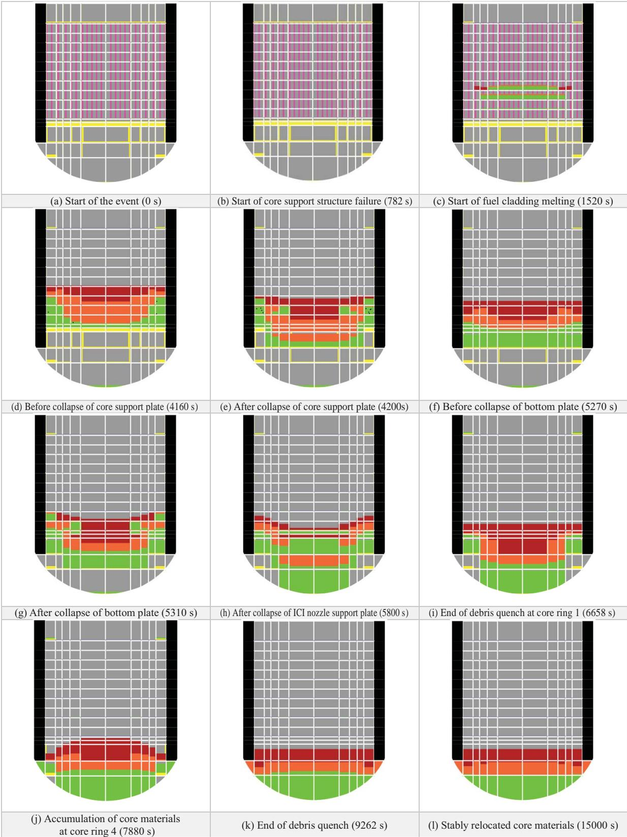
**Figure 4. Core degradation behavior**
