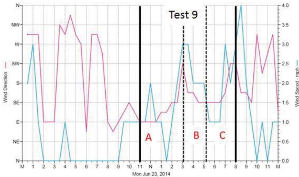
Figure 13 – Outside wind direction and speed for Test 9.
