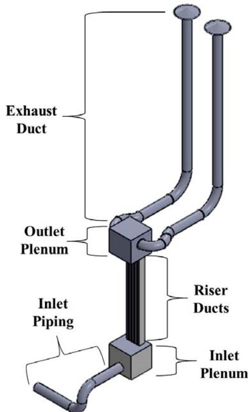
Figure 2 – Solid model rendering of UW quarter-scale air RCCS.
