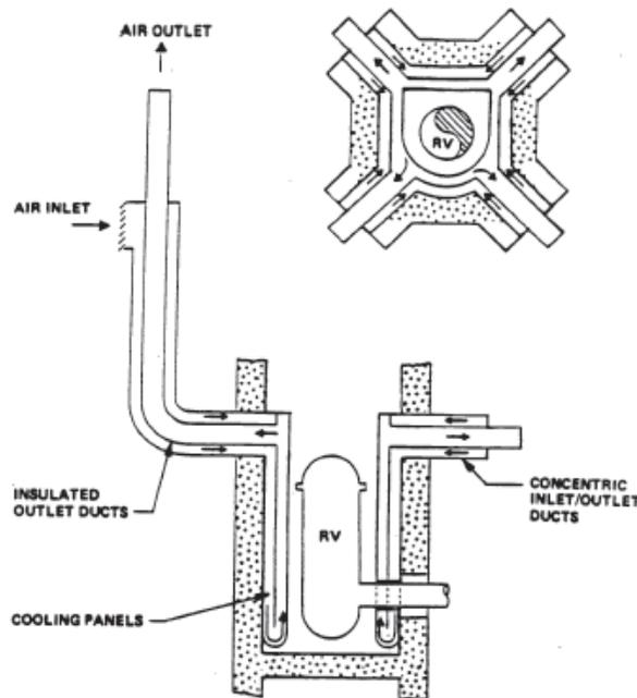
Figure 1 - Cavity plan view of RPV and RCCS.<sup>2</sup>
