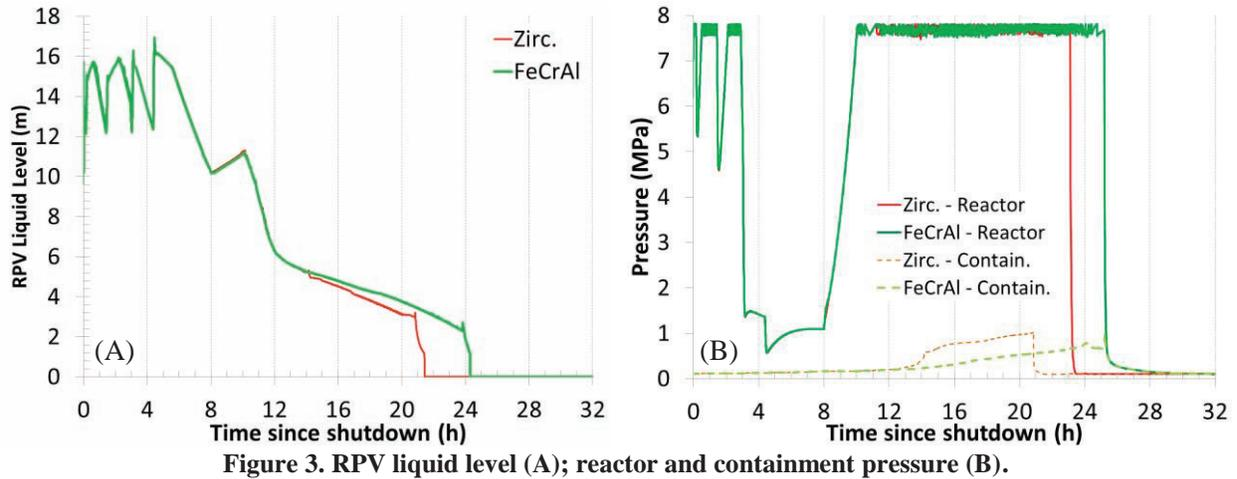
Figure 3. RPV liquid level (A); reactor and containment pressure (B).
