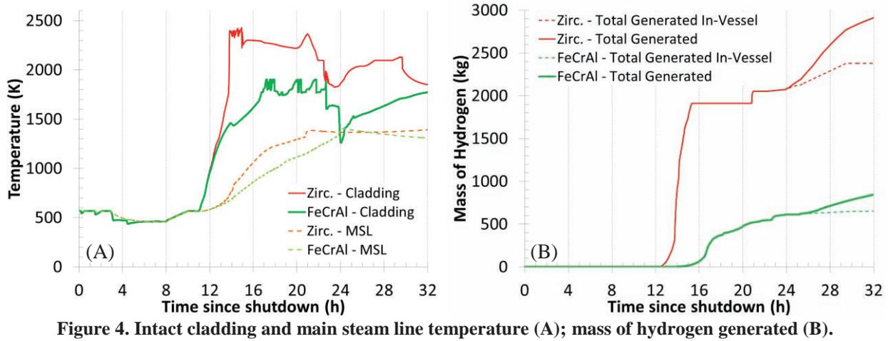
Figure 4. Intact cladding and main steam line temperature (A); mass of hydrogen generated (B).
