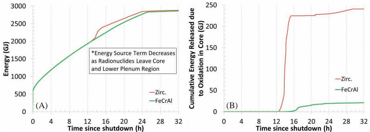
Figure 5. Total cumulative energy generated in core (A); cumulative energy from oxidation in core (B).
