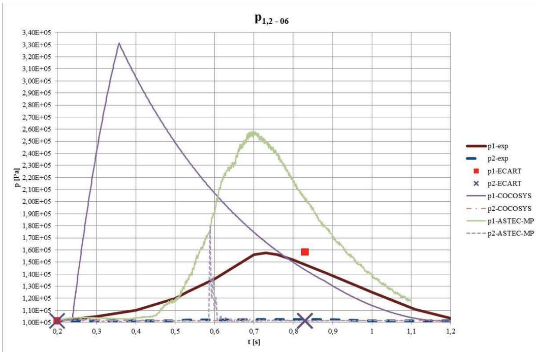
Figure 7. Pressure transients (test 06: exp. and simulations results).
