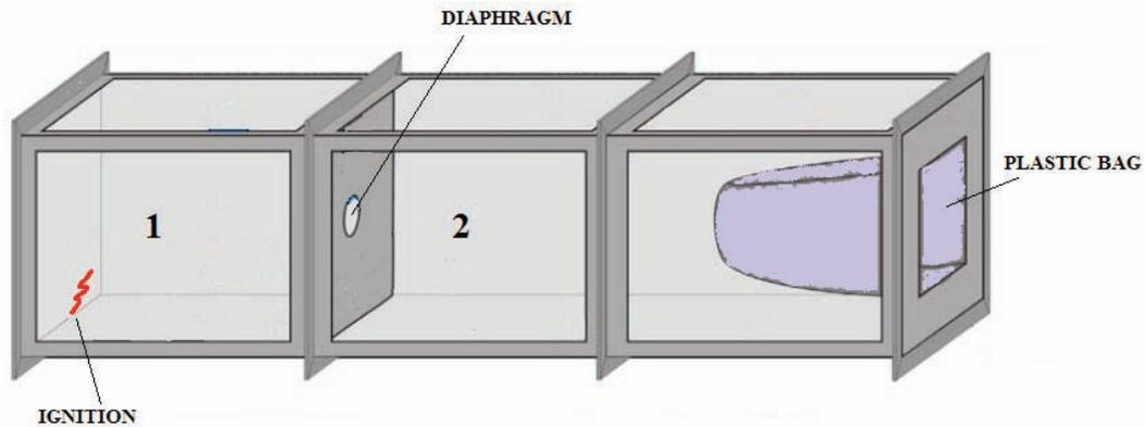
**Figure 1. LargeView2 apparatus vessel.**
