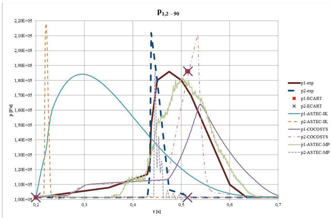
Figure 5. Pressure transients (test 90: exp. and simulations results).
