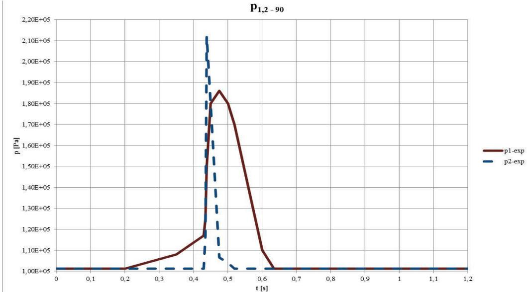
Figure 2. Pressure transient of test 90.
