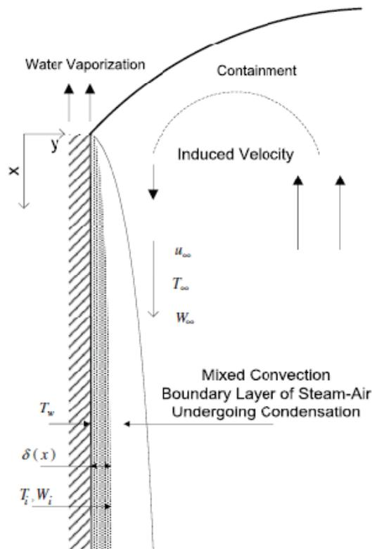
Figure 2. Flow pattern and the wall heat removal model
