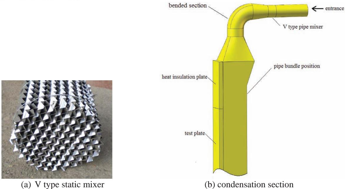
Figure 5. Entrance mixer and eliminating turbulent structure
