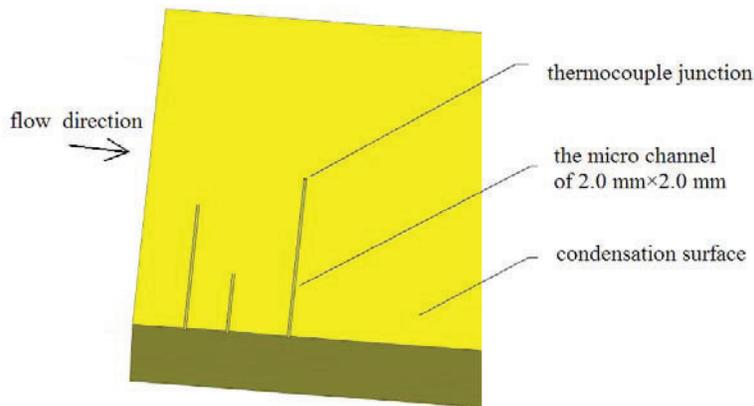
**Figure 8. Thermocouple arrangements**
