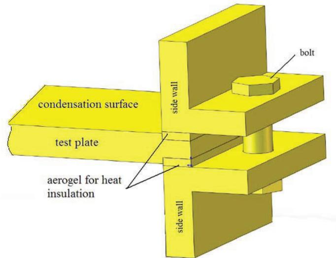
Figure 6. Test plate isothermal method
