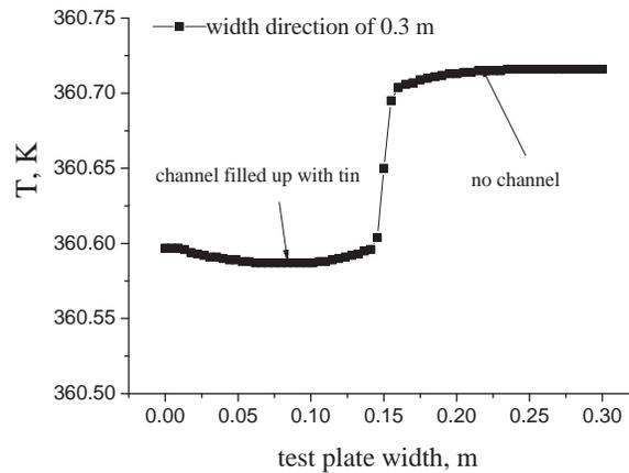
**Figure 9. Temperature profiles by tin filler on condensation side**
