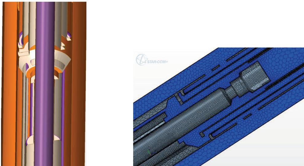
Figure 1: Geometry damper, bypass, labyrinth, piston (left). Volume mesh detail labyrinth (right)
