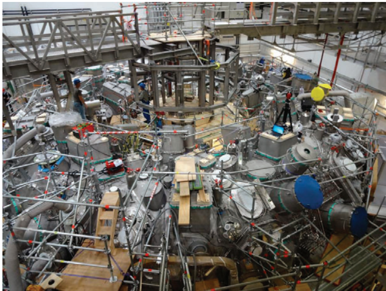
Figure 1. Picture of torus of W7-X facility which is under construction taken at the end of 2013.
