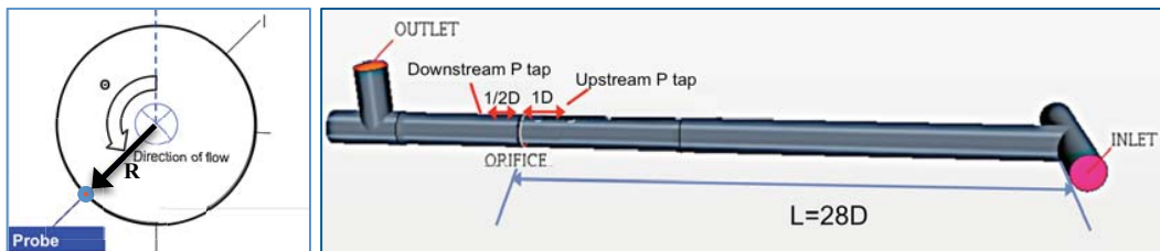
Figure 2: Angular location of pressure taps (left) and geometry of the experimental test (right)
