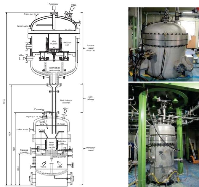
**Figure 12. Experimental setup.**
