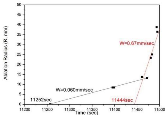
Figure 10. VESTA-S test results on the ablation rate.
