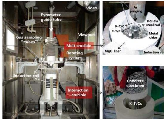
Figure 9. VESTA-S test facility.
