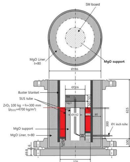
Figure 7. Jet impingement test section.
