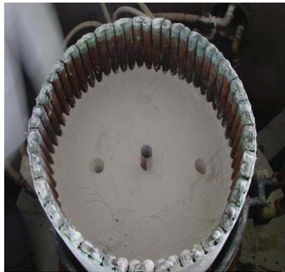
Figure 2. Charging of  $\text{ZrO}_2$ .
