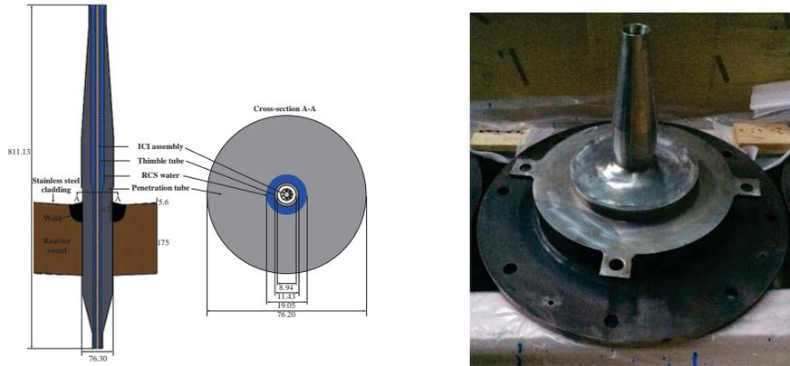
**Figure 11. APR1400 in-core-instrumentation penetration tube and test specimen.**
