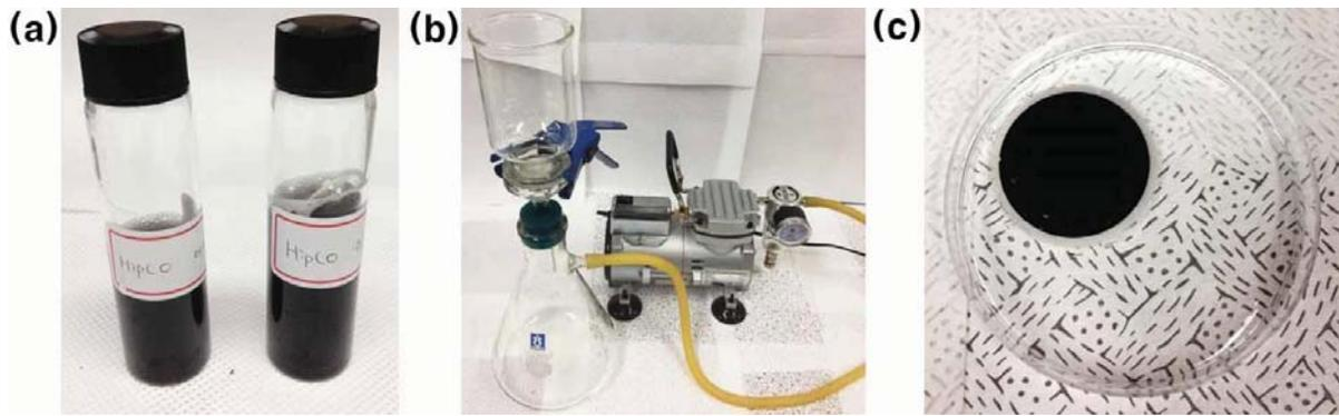
**Figure 3. (a) Dispersed HiPco CNT solutions; (b) Vacuum filtration equipment for the synthesis of randomly oriented CNT network film; (c) CNT film with a supporting substrate.**
