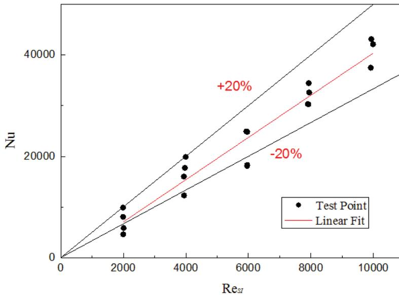
**Figure 8. Experimental relationship between Nusselt number and safety injected Re number: mist flow in water-injected**
