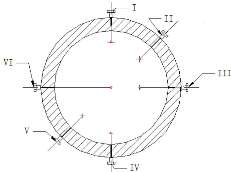
Figure 3. Cross-section with thermocouple
