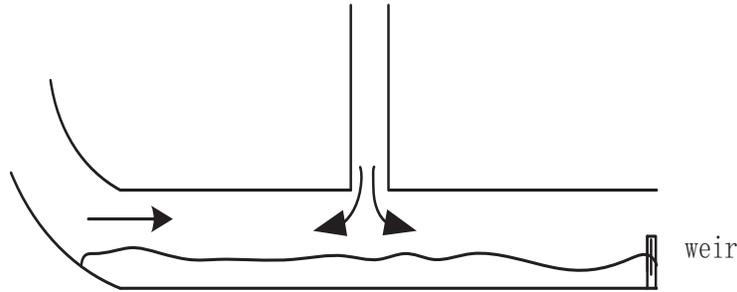
**Figure 4. Schematics of flow regime and condensation in COSI experiment.**
