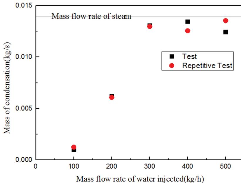
**Figure 9. Mass flow rate of water injected effected on condensation**
