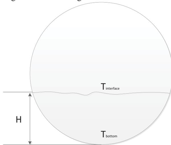
**Figure 6. Cross section of cold leg near after condensation**
