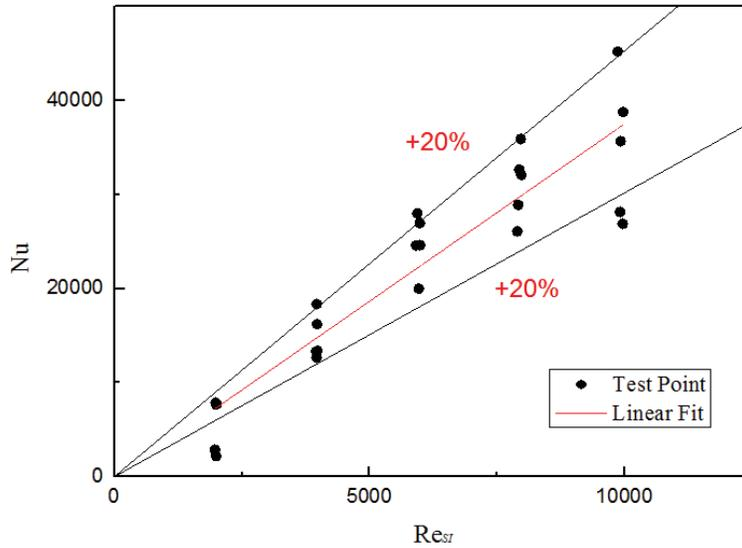
**Figure 7. Experimental relationship between Nusselt number and safety injected Re number: steam flow in water-injected**
